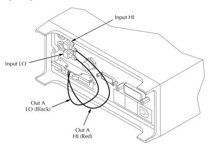
For 4-pole operation, connect OUT A HI (red) to INPUT HI and connect OUT A LO (black) to INPUT LO. Also connect OUT B HI (red) to SENSE HI and connect OUT B LO (black) to SENSE LO. See Figure 2-11.
