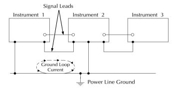
Figure 3-7 shows how to connect several instruments together to eliminate this type of ground loop problem. Here, only one instrument is connected to power line ground. Ground loops are not normally a problem with instruments having isolated LO terminals. However, all instruments in the test setup may not be designed in this manner. When in doubt, consult the manual for all instrumentation in the test setup.
