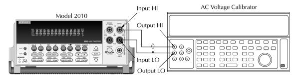
Figure 2-6 Function generator connections for manufacturing calibration (firmware revision A14 and higher)
