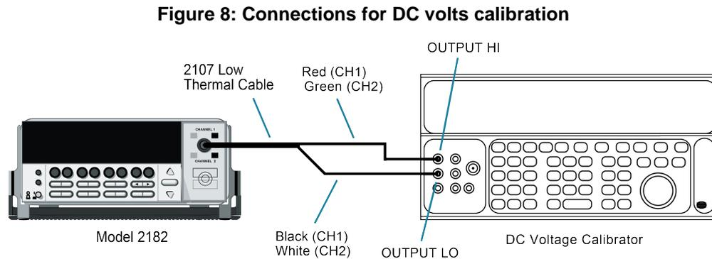
The Model 2107 cable connections are summarized in the following table.
