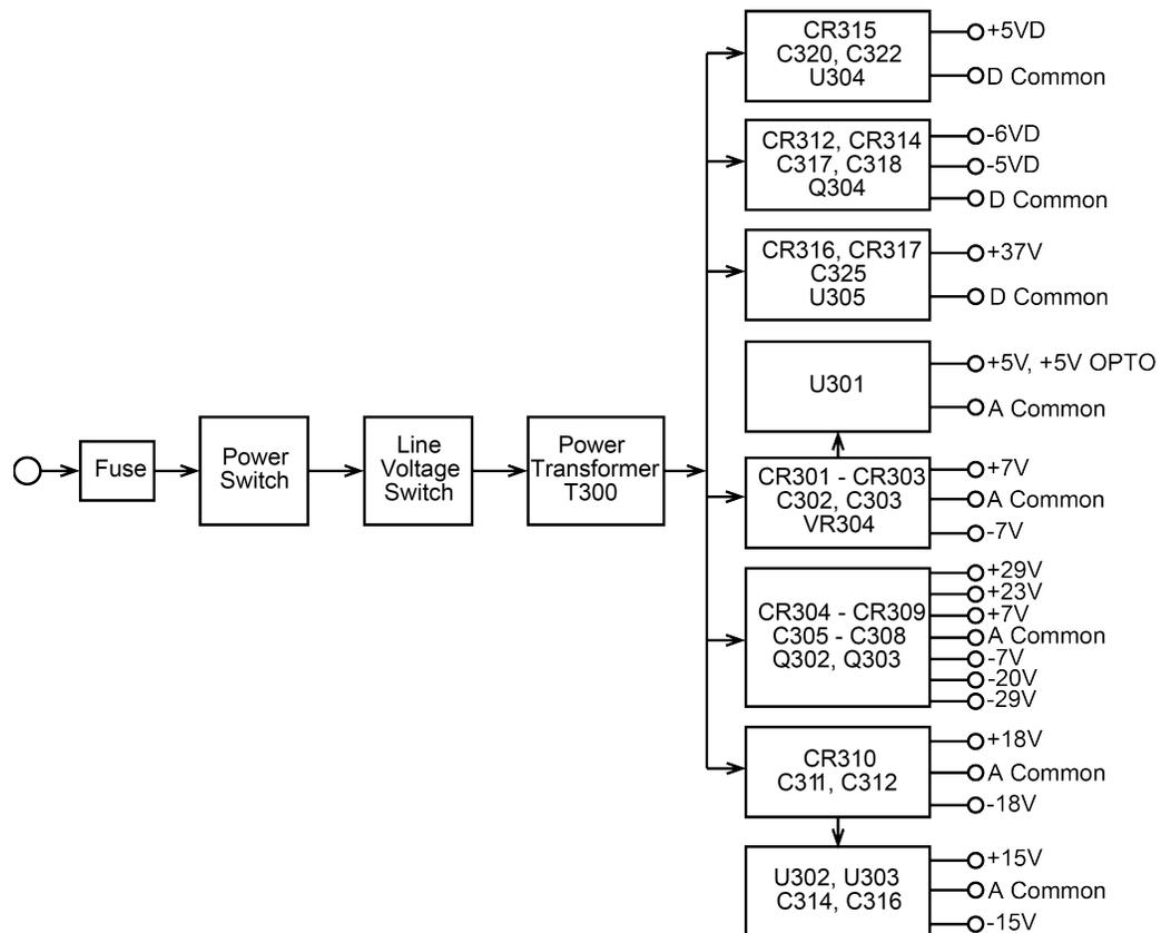
AC power is applied to the ac power module receptacle. Power is routed through the line fuse and line voltage selection switch of the power module to the power transformer. The power transformer has several secondary windings for the various supplies.
