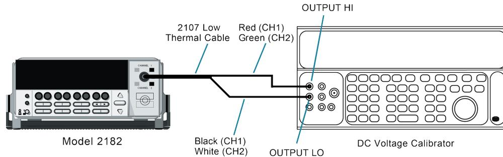
Connections for the Model 2107 Low Thermal Input Cable are summarized in the following table.
