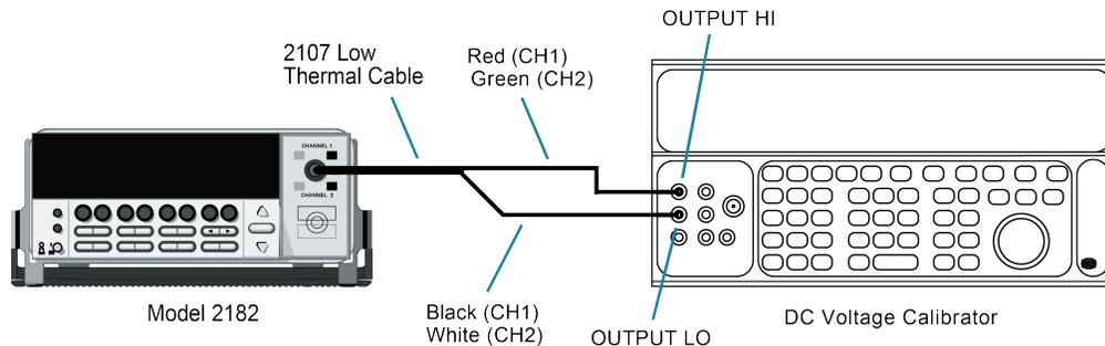
The Model 2107 cable connections are summarized in the following table.
