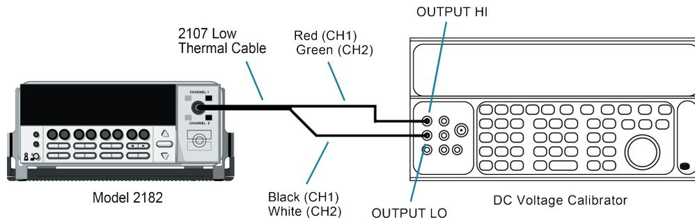
Figure 9: Connections for DC volts calibration
