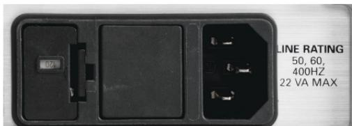
3. Connect the plug of the power cord to a grounded ac outlet.
