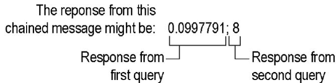
If a command or query has the same root and lower-level nodes as the previous command or query, you can omit these nodes. In the following figure, the second command has the same root node (STAT:QUES) as the first command, so these nodes can be omitted.
