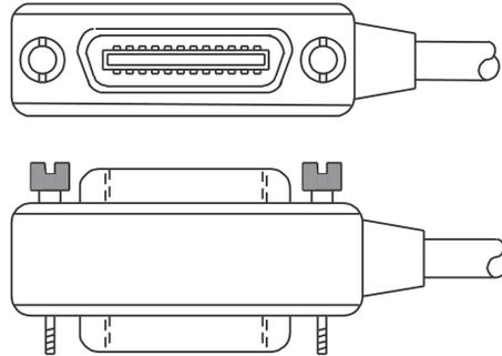
To allow many GPIB connections to other instruments, stack the cable connectors. Two screws are located on each connector to ensure that connections remain secure. The figure below shows a typical connection scheme for a multi-unit test system.
