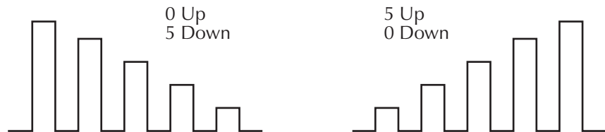
Figure 3-6 Sample one-shot only pulses for step method
