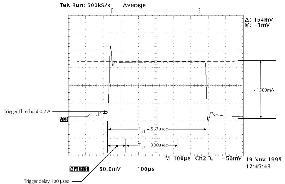
**NOTE** In Figure 6, a trigger delay of 100 $\mu$ s is used to eliminate the effect of a current transient on the pulse current measurement.
