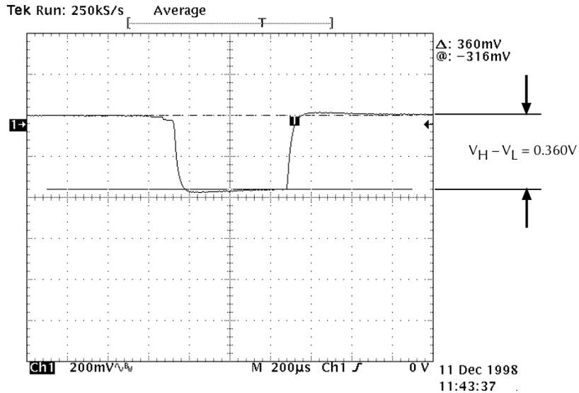
**NOTE** *Figure 15 shows the voltage drop during the transmit portion of the pulse of a GSM phone using the Model 2306 battery channel with output impedance set to 0.24Ω. See Figure 14 for actual Li ion battery results.*
