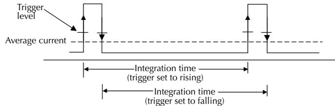
**NOTE** The pulse waveform contained in Figure 8 shows trigger level and the integration time used by the Model 2306 for pulse current measurements.
