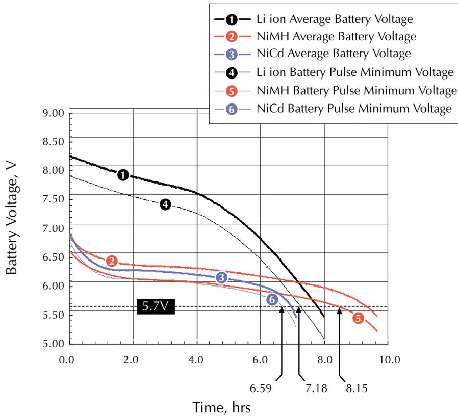
**NOTE** Figure 10 shows the average and minimum battery pack terminal voltage during a load pulse from a dynamic load simulating a GSM phone.
