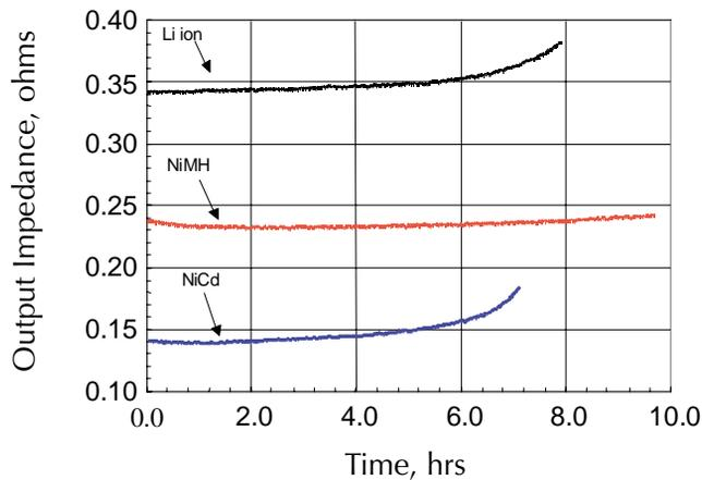
**NOTE** *Figure 12 shows electronic resistance for battery packs during a simulated GSM phone pulsed discharge from full charge to 5.5 volts.*
