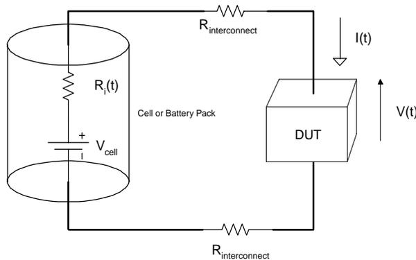
If  $R_{\text{interconnect}}$  is small compared to  $R_i(t)$  and if  $R_i(t)$  is relatively constant during the length of the pulse,  $R_i(t) \sim R_i$ , then the voltage across the DUT may be expressed as:
