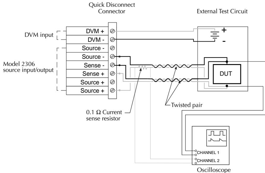
**NOTE** Figure 7 contains a simple circuit for determining the dynamic voltage and current characteristics of the DUT using a 2-channel oscilloscope, a 0.1 ohm resistor used as a current sense resistor, and a voltage probe at the DUT.
