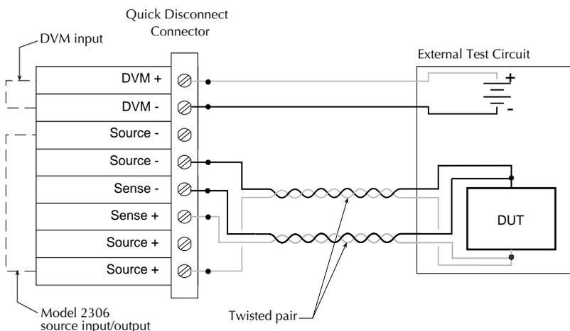
**NOTE** DO NOT jumper the sense inputs and supply outputs at the rear of the supply.
