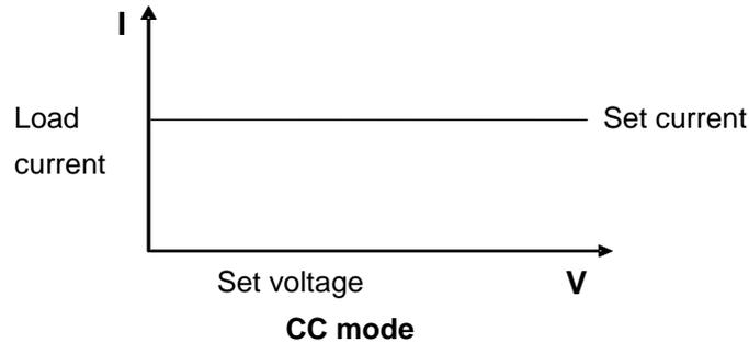
Figure 5 Voltage-current relation under CC Mode
