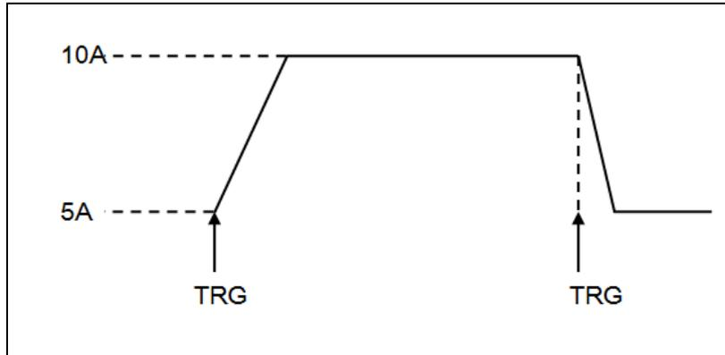
Figure 11 Dynamic test in toggle mode
