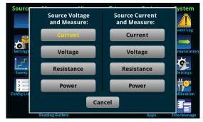
The instrument saves many of the settings with the source or measure function that was active when you set them. For example, if you set the measure function to current and you set a value for NPLCs, the instrument saves the NPLC value for that measure function. When you change the measure function to voltage, the NPLC value changes to the value that was last set for the voltage measure function.
