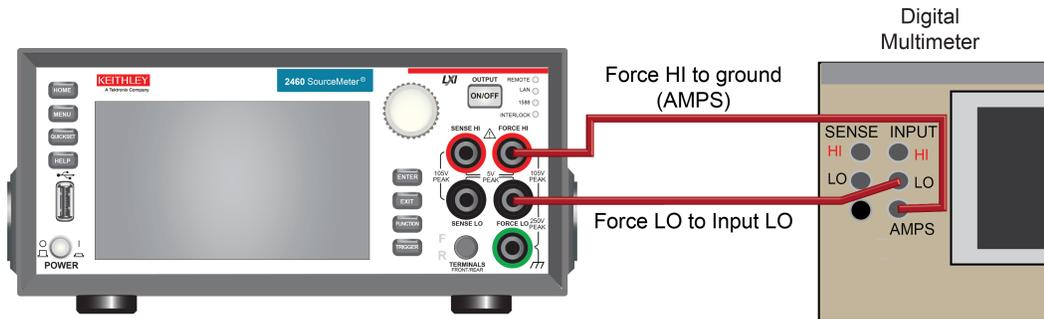
**Figure 4: Rear-panel connections for the 1  $\mu$ A to 1 A ranges**
