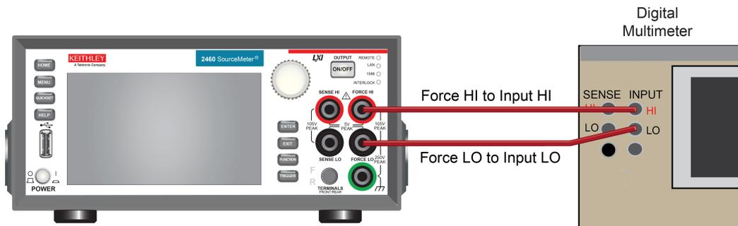
**Figure 2: Rear-panel connections for the 200 mV to 100 V ranges**
