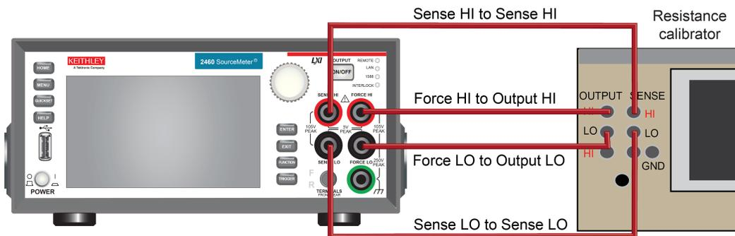
**Figure 8: Rear-panel resistance connections**
