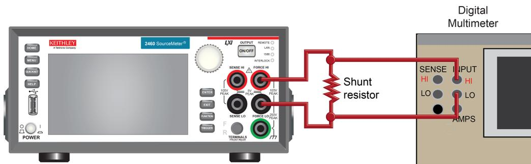
**Figure 6: Rear-panel connections for the 4 A to 10 A ranges**
