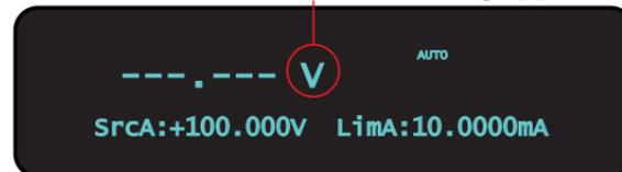
2. Press the **AUTO** key as many times as needed to select the AUTO range function. When AUTO is selected, the 2657A automatically selects the best range for the measured value. You will briefly see the display shown below, and then the main display screen reappears.
