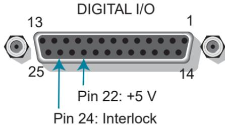
A  $+5.0$  V pin is also available on the digital I/O connector (pin 22). To use the interlock, connect the 5 V pin and the interlock pin to the input and output, respectively, of the switch in your test system.
