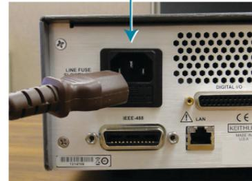
3. Connect the plug of the power cord to a grounded ac outlet.
