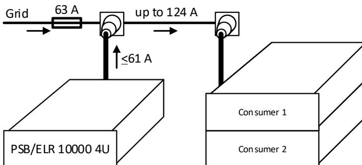
When running a higher number of recovering, i. e. energy backfeeding units on the same leg of the installation, the total currents per phase increases accordingly.
