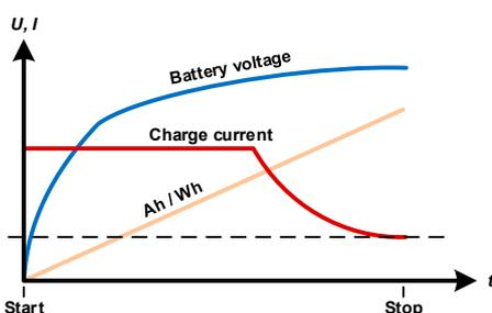
The fourth mode is called **Dynamic test** and combines **Static discharge** with **Static charge** in one flow. The same parameters for the single test parts are available, plus some extra for the flow. You can, for example, select what comes first, charge or discharge. There is also an option to cycle the test, i. e. repeat 1 to 999 times or infinitely and you can define a resting period which elapsed before the next cycle.
