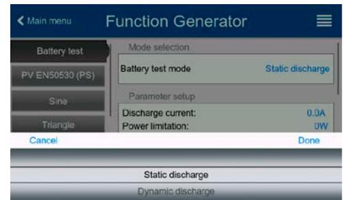
There is a choice of modes: **Static discharge** (constant current), **Dynamic discharge** (pulsed current), **Static charge** (constant current) and **Dynamic test** (flow of charge/discharge).
