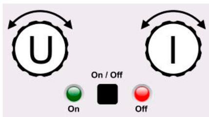
The physical quantities on the depiction of the knob show the current assignment. The left knob is always assigned to the voltage (U), while the right knob can be switched by tapping on the depiction. Furthermore, the DC terminal status is indicated by two LEDs (green = on).
