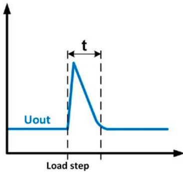
Example for a neg. load step: the DC output will rise above the adjusted value for a short time.  $t$  = transient time to settle the output voltage.
