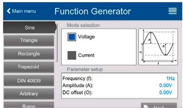
2. In the menu select the desired function by tapping on the list on the left-hand side. Depending on the choice of function there follows a request to which value the function generator is going to be applied, **Voltage** or **Current**.
