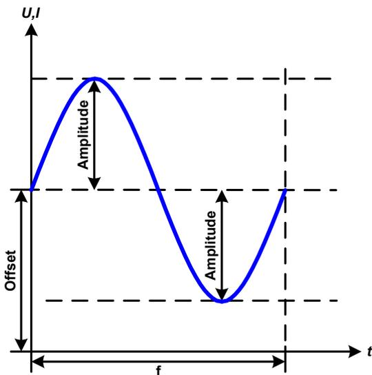
A normal sine wave signal is generated and applied to the selected set value, e.g. current (I). At a constant input voltage the current input of the load will follow a sine wave.
