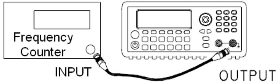
2. Set the instrument to the output (found in the table below) and measure the output frequency. Be sure the instrument output is enabled.
