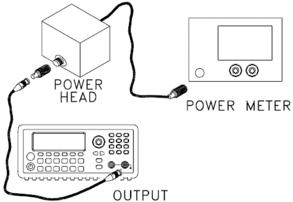
Connect the power meter to measure the output amplitude of the instrument as shown below.
