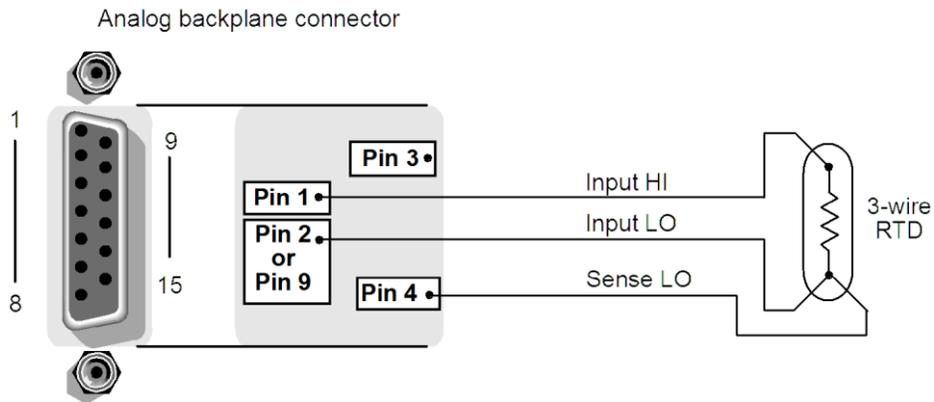
**Figure 5-38: Three-wire RTD switching module connections**
