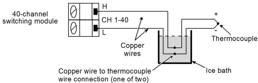
**Figure 5-34: Internal reference junction (40 channel switching module)**
