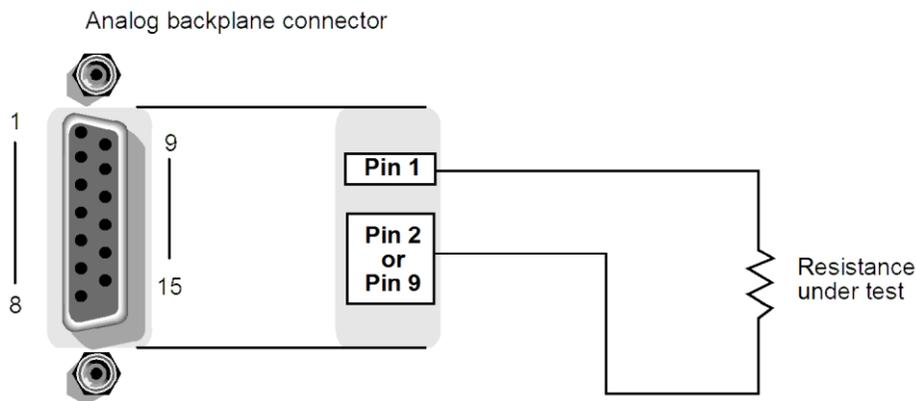
Connections to test continuity using a switching module are shown below. Because this is a 2-wire ohms measurement, Channels 1 through 40 of a 40-channel switching module can be used.
