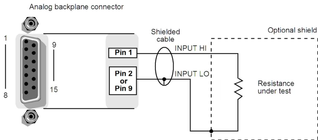
**NOTE** Source current flows from the connector HI to the connector LO pins.
