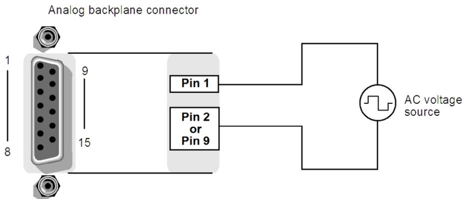
**Figure 5-42: FREQ and PERIOD connections (switching module)**
