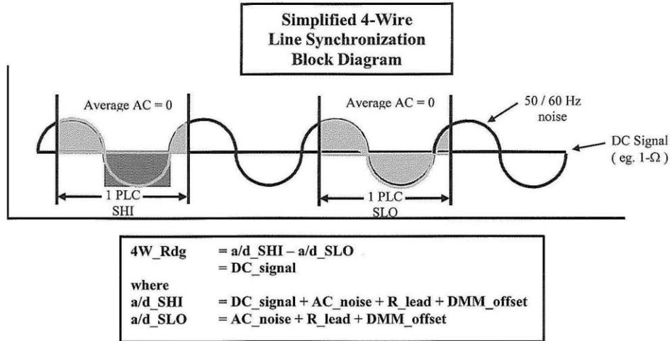
For Line Synchronization off and  $<1plc$ , reading rate increases, but measurement uncertainty and noise increases due to the Average AC noise during the SHI phase not cancelling with the SLO phase. With Line Synchronization ON, the SHI and SLO measurement phases are triggered at the rising edge of the power line zero crossing. This improves reading uncertainty and noise by  $>30x$  while minimal reading rate reduction.
