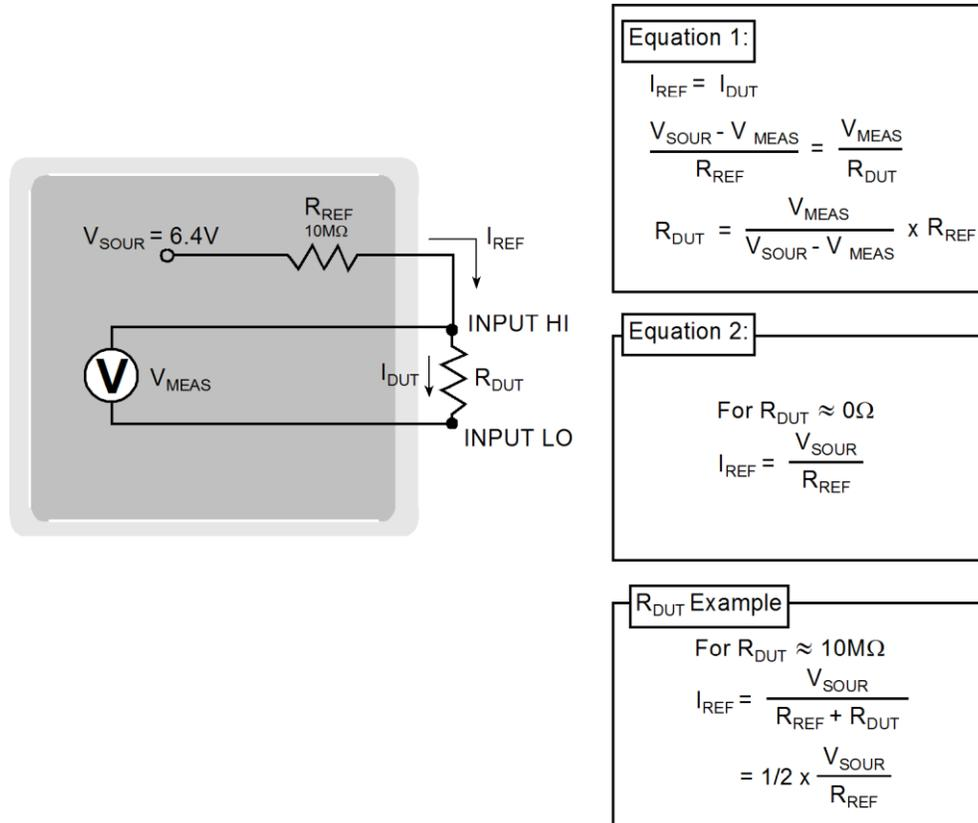
Because  $I = V/R$ , Equation 1 is modified using the  $V/R$  equivalents in place of  $I_{REF}$  and  $I_{DUT}$ . Therefore:
