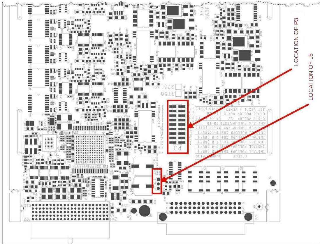
The connector labeled P3 contains all of the jumpers needed to configure digital I/O and VEXT1, VEXT2. The connector labeled J5 contains a single jumper option that configures the backplane relays. See the following table for individual jumper locations and effects.
