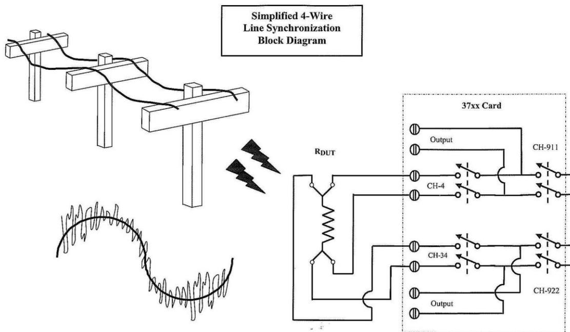
Traditional DMM 4-wire measurements are made in two phases, SHI and SLO. If the `dmm.nplc=1` or a multiple of the power line, theoretically, the average AC noise is 0. Refer to the 4W-Rdg calculation ([http://www.maxim-ic.com/appnotes.cfm/appnote\\_number/1041/](http://www.maxim-ic.com/appnotes.cfm/appnote_number/1041/)).
