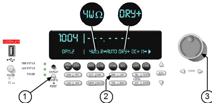
**NOTE** The Series 3700 is in 4-wire ohm mode when the 4WΩ is displayed. Dry Circuit is active when the DRY+ is displayed (see the above figure).
