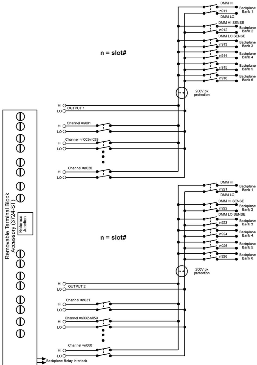
Figure 9-40: Models 3720, 3723, and 3724 screw terminal
