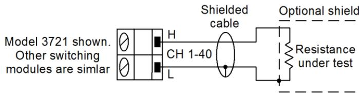
For  $4W\Omega$  measurements, a channel pair is used for each 4-wire measurement as shown. For  $4W\Omega$  connections on a 40-channel switching module, Channels 1 through 20 (which are used as the INPUT terminals) are paired to Channels 21 through 40 (which are used as the SENSE terminals). Channel 1 is paired to Channel 21, Channel 2 is paired to Channel 22, and so on.
