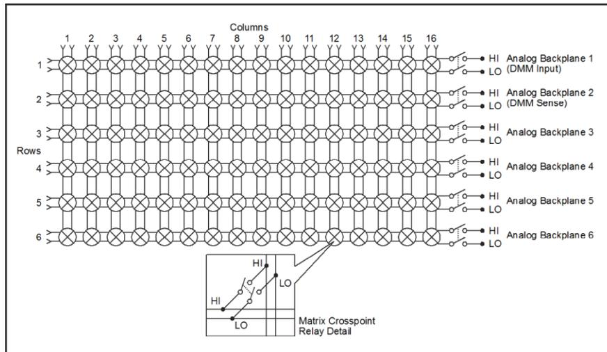
The channels on the 3730 are matrix channels. Unlike MUX channels, matrix channels do not have a DMM configuration associated with them. Therefore, specifying a matrix channel in the channel list parameter to the `dmm.setconfig()` function generates an error. To connect a DMM configuration to matrix channels, create a channel pattern with desired channels and analog backplane relays.
