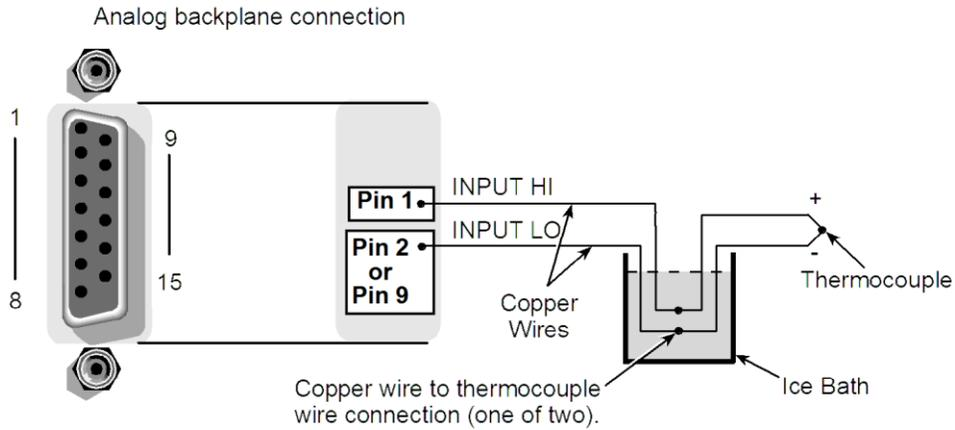
**NOTE** The positive lead of the type T thermocouple is made of copper. Therefore, that lead can be connected directly to the input of the switching module (it does not have to be maintained at the simulated reference temperature, in other words, immersed in an ice bath).
