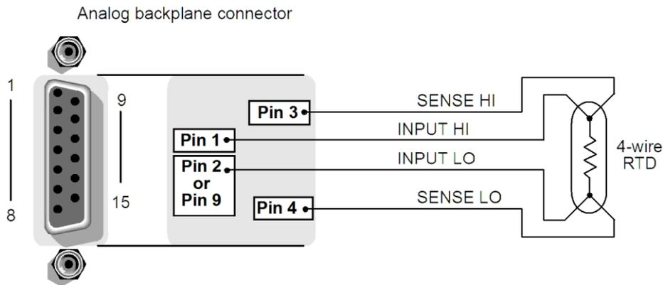
Figure 5-40: Four-wire RTD switching module connections
