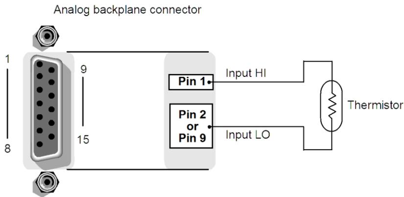
**Figure 5-36: Thermistor switching module connection**
