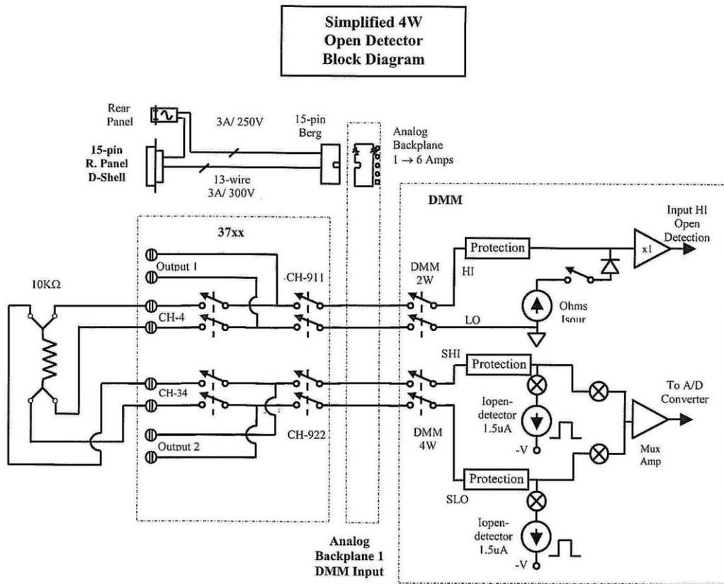
Figure 5-28: Model 3706 Internal DMM
