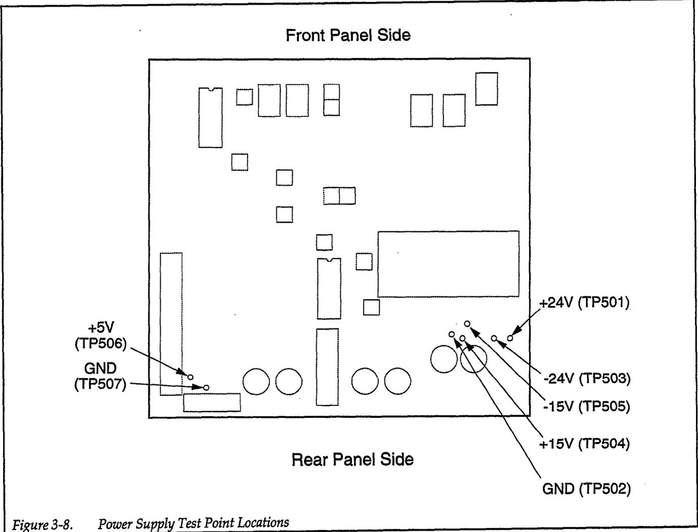
Figure 3-8. Power Supply Test Point Locations
