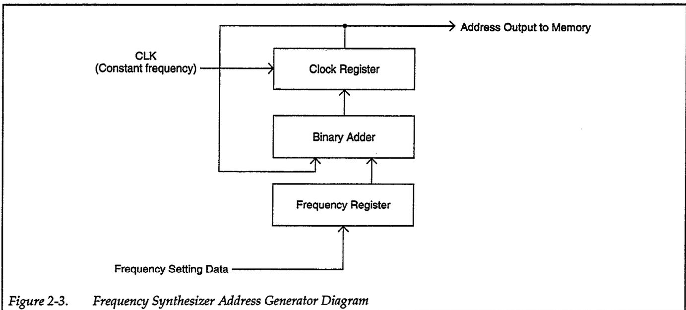
Figure 2-3. Frequency Synthesizer Address Generator Diagram
