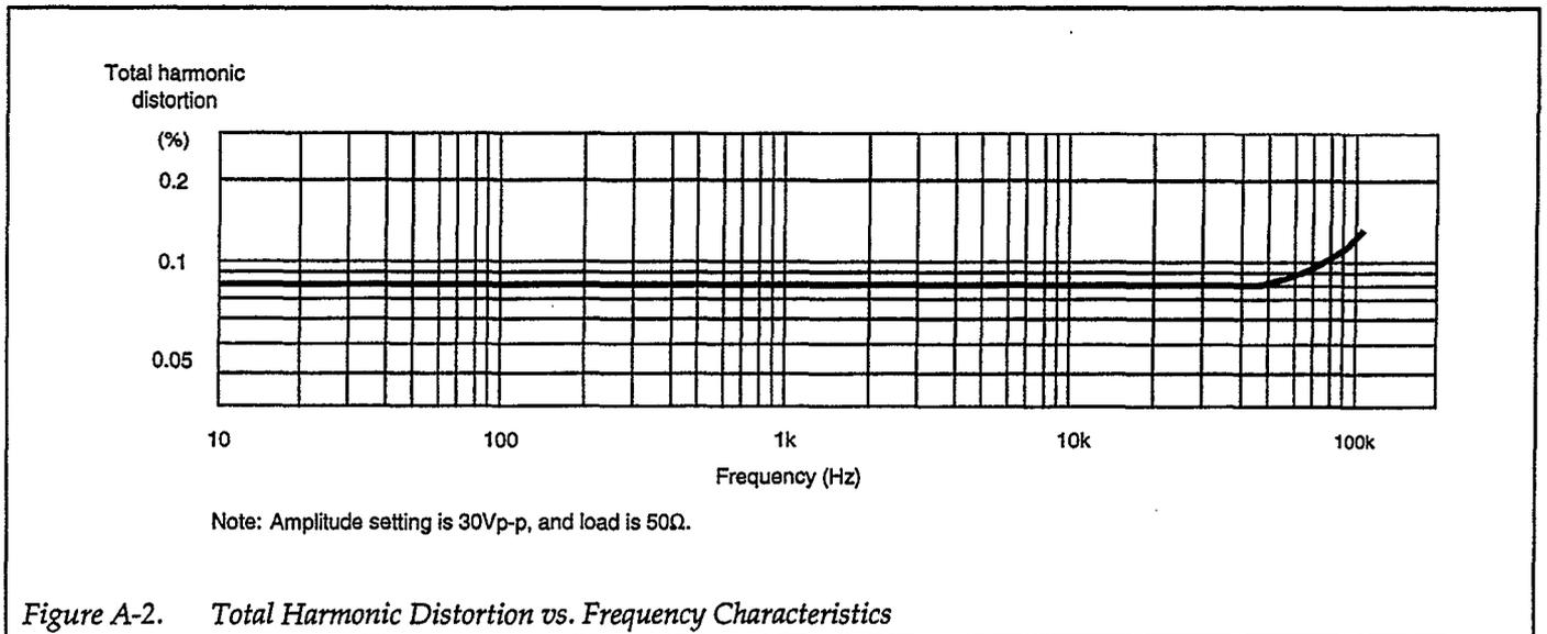
Figure A-2. Total Harmonic Distortion vs. Frequency Characteristics
