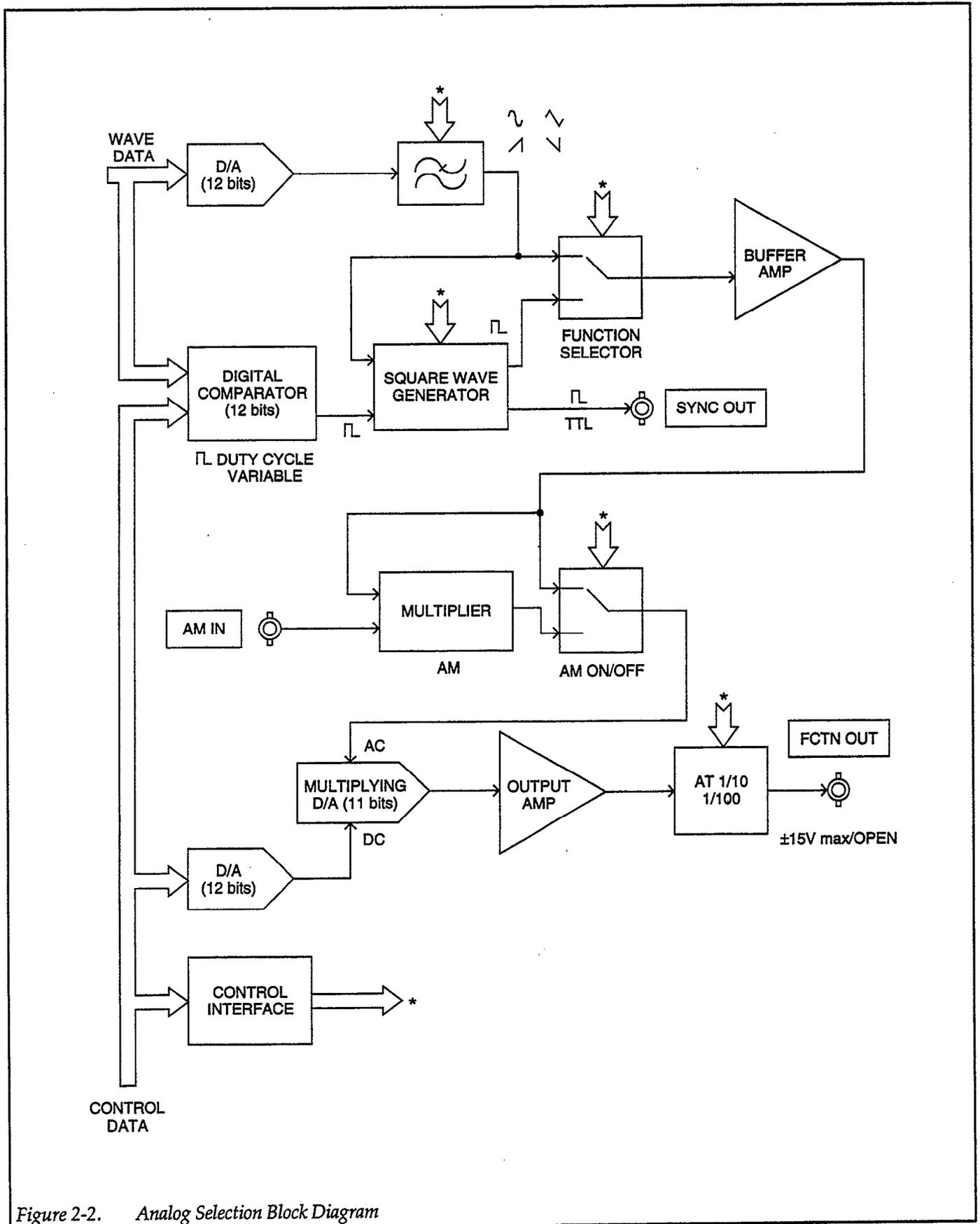
Figure 2-2. Analog Selection Block Diagram
