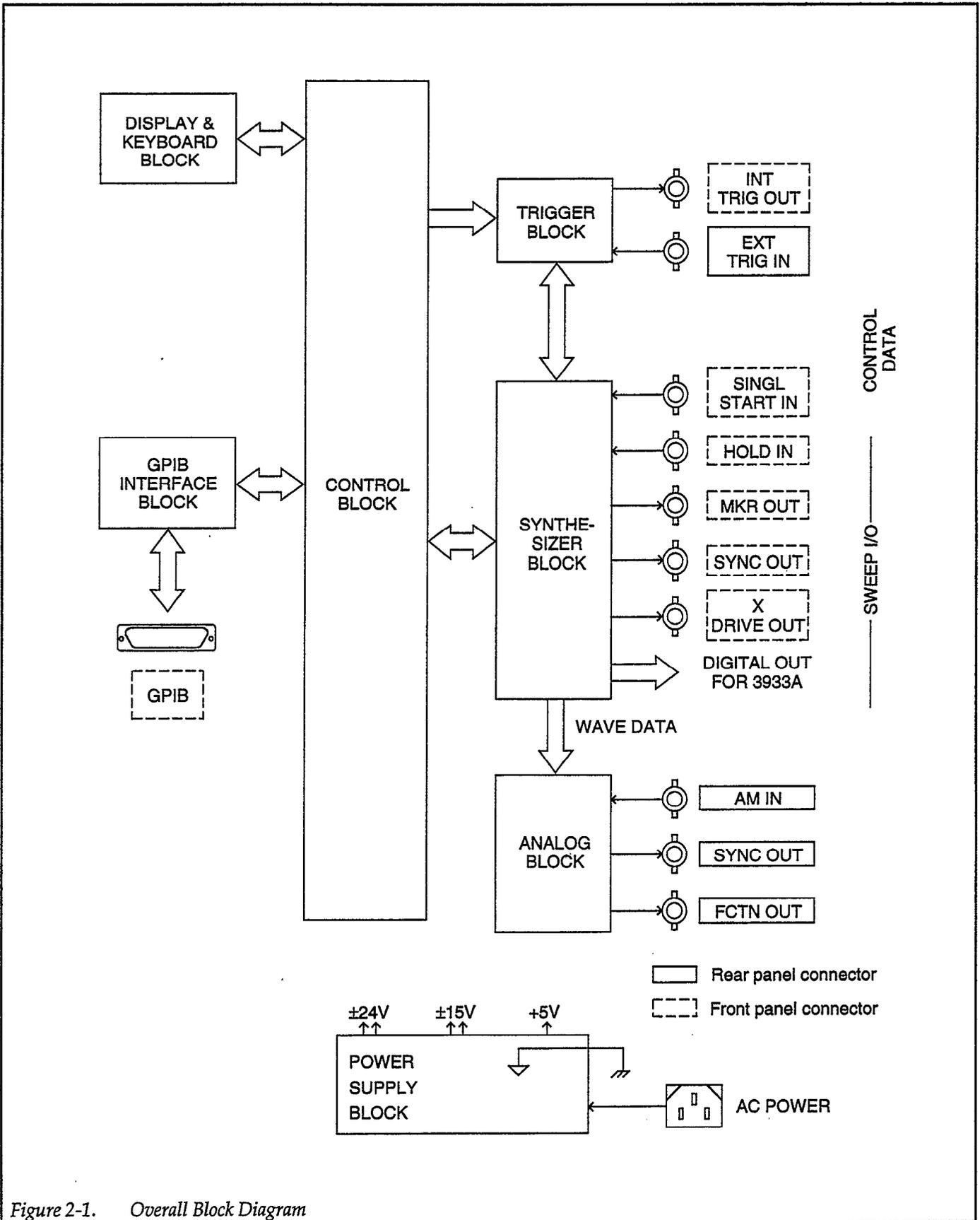
Figure 2-1. Overall Block Diagram
