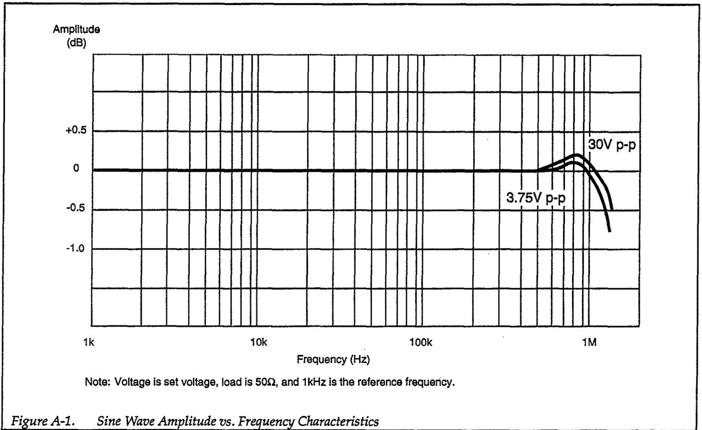
Figure A-1. Sine Wave Amplitude vs. Frequency Characteristics
