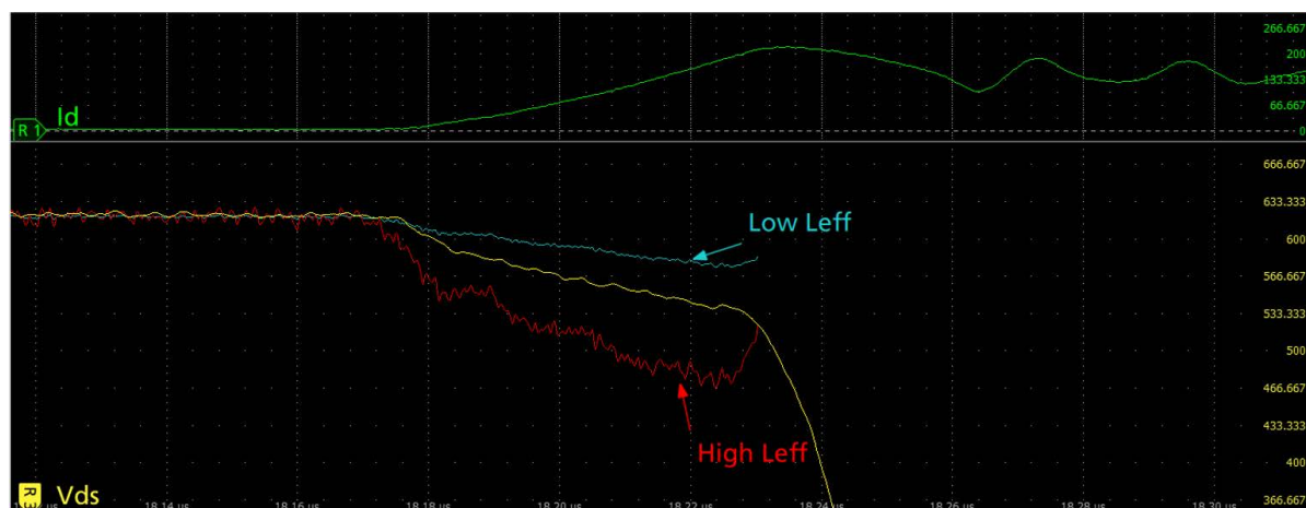
Figure 43: V_{\text{ds}} modelled using low L_{\text{eff}} (blue) and high L_{\text{eff}} (red) to match zero skew acquired V_{\text{ds}} (yellow) during turn on transient
