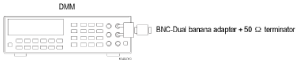
Figure 3: 50 Ω terminator accuracy
