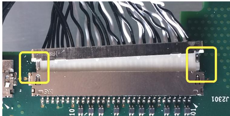
7. Repeat these steps to disconnect the remaining smaller cable connector.
