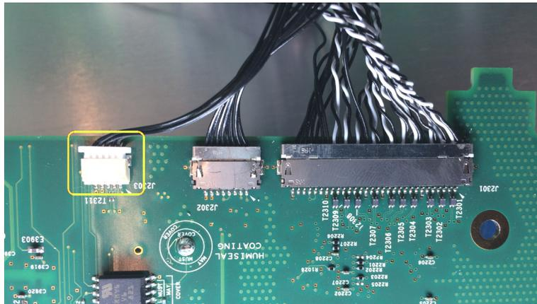
5. Position your fingernails so that they are between the edge of the larger-size cable connector and its board connector.
