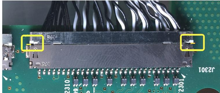
6. Gently push and rock the cable connector side to side to move the wire connector out of the board connector.
