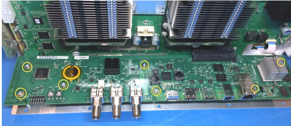
2. Lift and pull the Processor board away from the chassis. It is still connected with cables, so be careful to not pull it too far.
