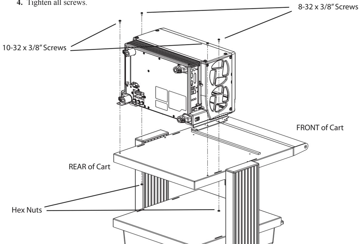
**Figure 5: Aligning Instrument With Cart, Shown On K420 Cart**
