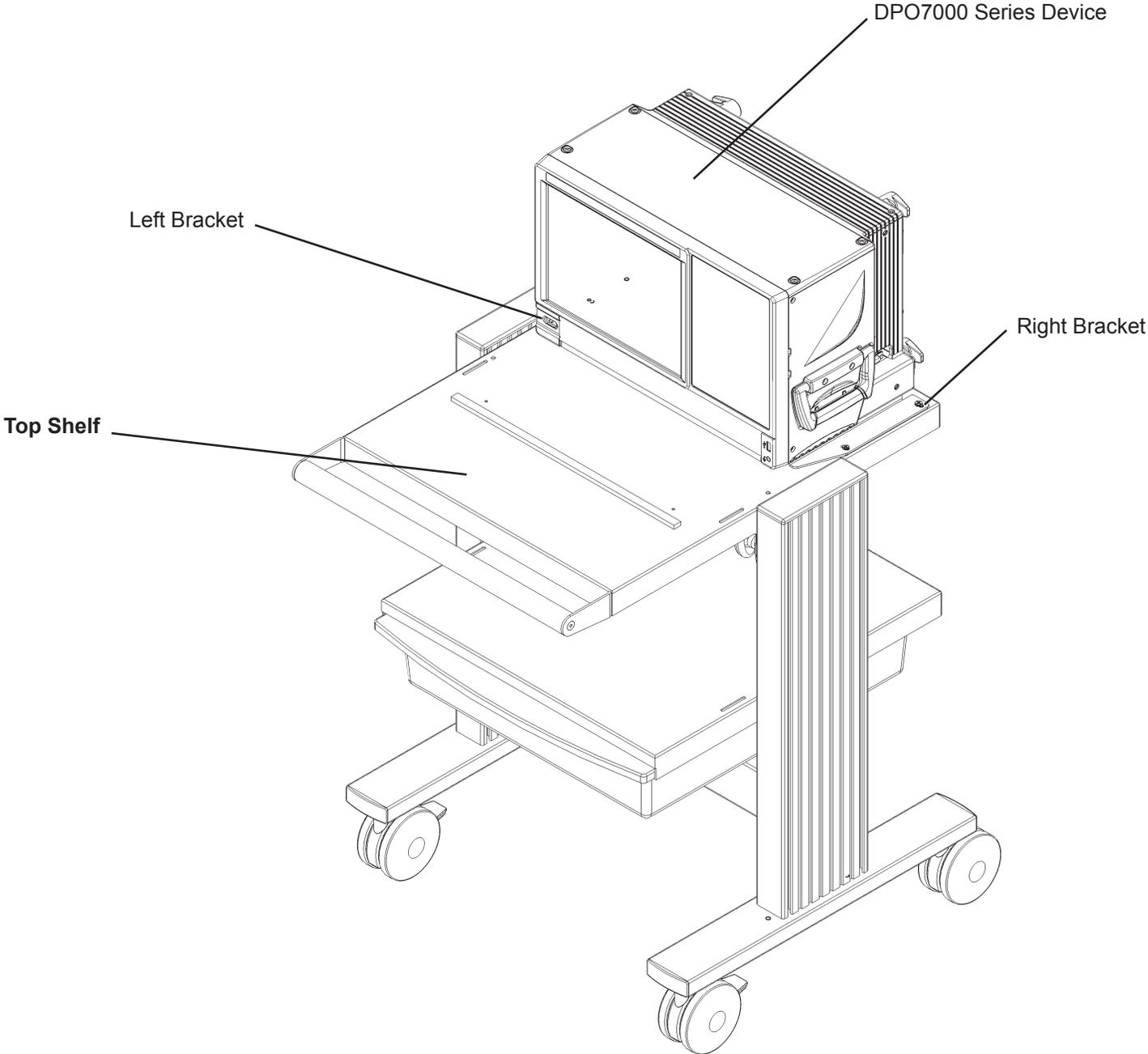
**Figure 2: Brackets & Device Shown On K420 Cart**
