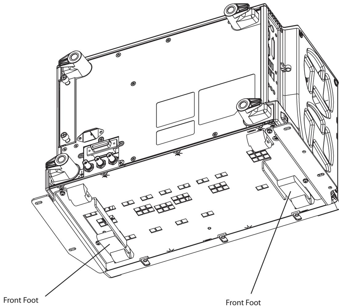
**Figure 4: Brackets Installed, Shown On DPO7000 Series Device**
