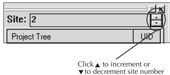
The title bar at the top of the KITE panel indicates which test is presently being displayed. In [Figure 4-37](#), test `vce-ic-2x` for Site 2 is displayed. The unique identifier (UID) distinguishes this test from any other test having the same name.
