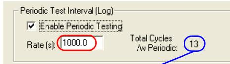
KITE calculates the Total Cycles /w Periodic: the total number of cycles: based on the Stress / Measure Cycle Times and the Periodic Test Interval. This value may not exceed 128.
