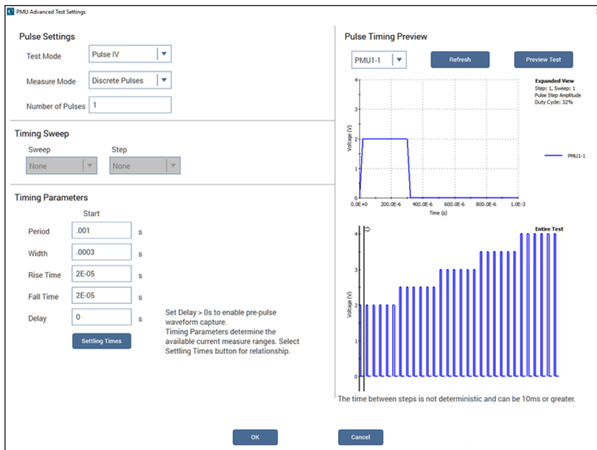
Figure 57: Six-point pulse amplitude sweep
