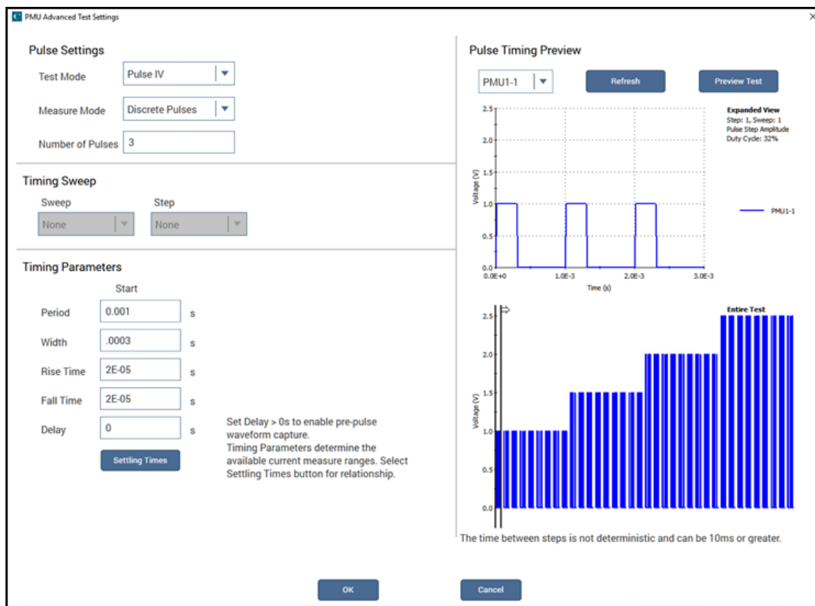
Figure 59: Two-channel test (stepping and sweeping) with three points (only PMU1-1 displayed)
