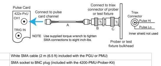
BNC socket to three-lug triaxial plug (included with the 4200-PMU-Prober-Kit)
