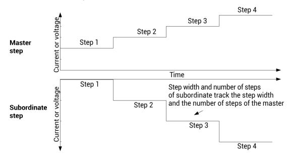
Figure 65: Master step versus subordinate step
