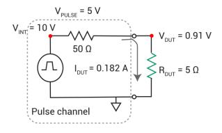
This figure shows a 5 V pulse into a 5  $\Omega$  DUT load.
