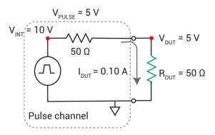
Example 1, showing a 5 V pulse into a 50  $\Omega$  DUT load.
