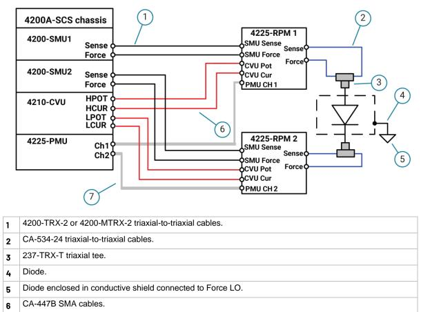
Figure 117: Connections from the 4200A-SCS and 4225-RPMs to the diode
