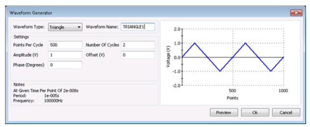
Figure 107: Triangle waveform
