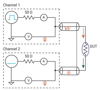
In the previous figure, the voltage pulse is applied by channel 1; channel 2 does not pulse. Therefore, there is no dV/dt, and therefore there are no charging or discharging currents during the pulse transition. The red arrows show charging and DUT current for channel 1. The green arrow illustrates the DUT current only for channel 2.
