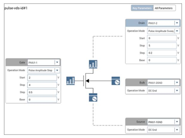
Figure 29: Key Parameters pane for the pulse-vds-id test
