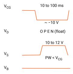
Figure 157: Program + Erase pulse waveforms for a floating gate DUT, with separate pulse waveforms for the DUT gate, drain, source, and bulk
