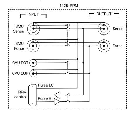
Figure 5: Wiring diagram of the RPM
