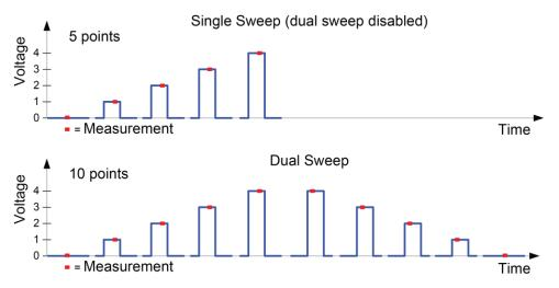
Figure 35: Single and dual pulse amplitude sweep examples
