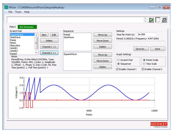
Figure 103: Custom File Arb operation: Copy waveforms into Sequencer
