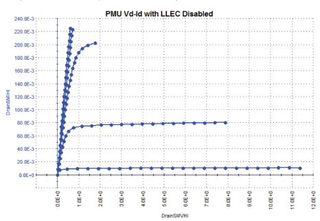
Figure 70: Vd-Id family of curves showing load-line effect (LLEC disabled)
