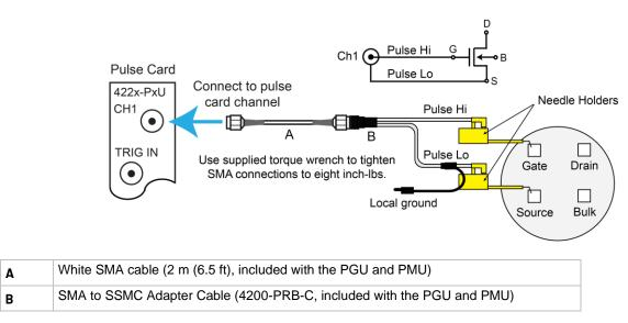
Figure 16: Pulse card connections using the SMA to dual SSMC adapter cable
