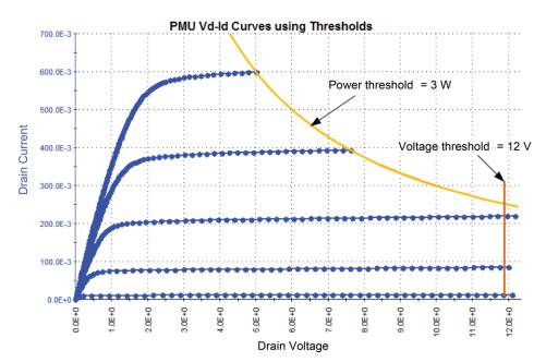
Figure 69: Vd-Id family of curves with LLEC disabled
