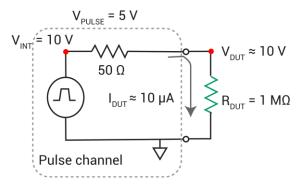
This example shows a 5 V pulse into a 1  $M\Omega$  DUT load.
