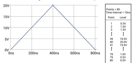
Figure 83: Full arb waveform example
