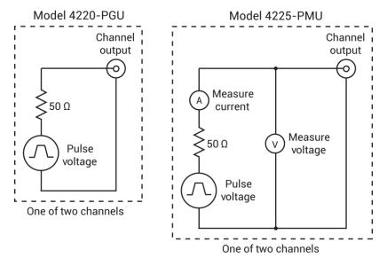
Figure 1: Simplified circuits of the PGU and PMU
