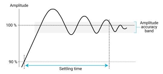
Figure 52: Settling time
