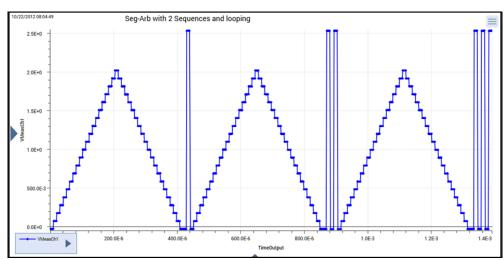
Figure 82: Graph of the waveform (two-sequence with looping) measurement
