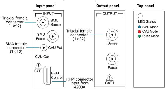
Figure 4: 4225-RPM panels
