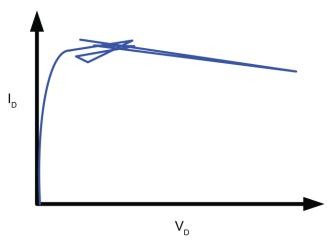
Figure 25: Curve showing poor LLEC compensation
