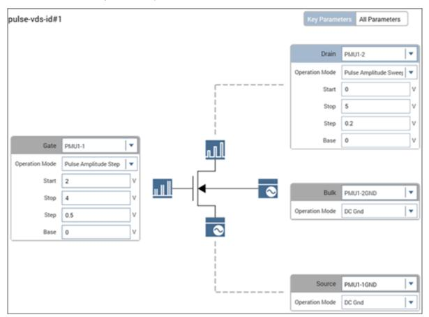
Figure 143: Key Parameters pane for the pulse-vds-id test
