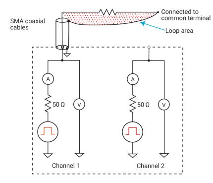
Figure 10: Two-terminal device connections to a pulse card using one channel
