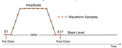
Figure 43: Waveform capture
