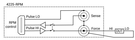
Figure 7: RPM wiring diagram for local sensing
