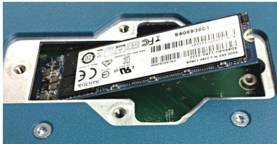
7. Grasp the edges of the raised end of the card and pull to remove the memory card. Store or destroy the memory card in accordance with your organization's guidelines.
