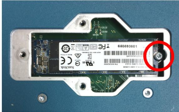
The end of the memory card lifts upward as you remove the screw.
