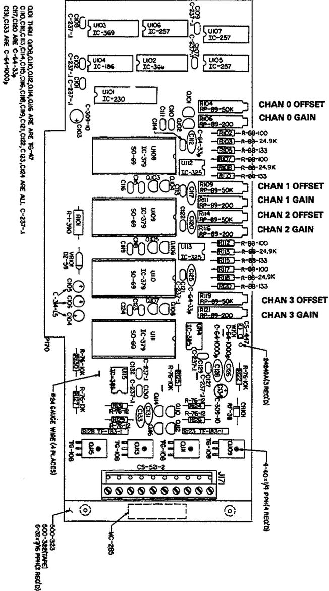
Figure 3. AOM4 Calibration Adjustments
