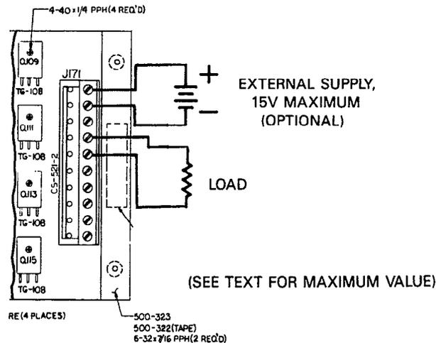
**Figure 2. Typical AOM4 Output Connections (Channel 0 shown)**
