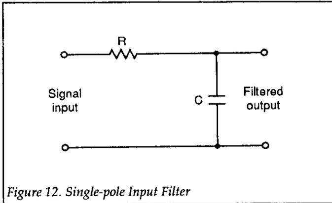
Figure 12. Single-pole Input Filter
