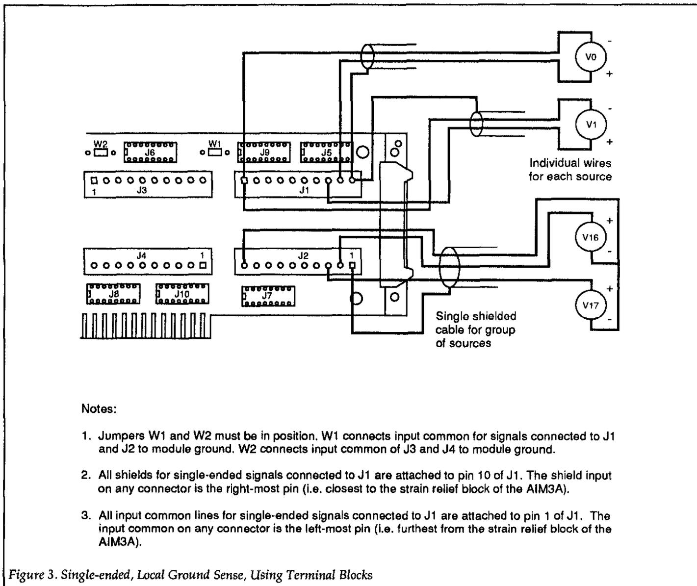
Figure 3. Single-ended, Local Ground Sense, Using Terminal Blocks
