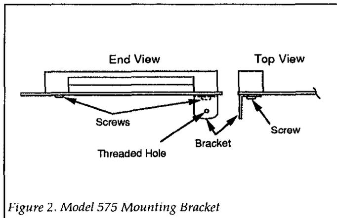
Figure 2. Model 575 Mounting Bracket
