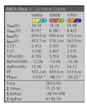
To add statistical readouts to individual measurement badges, double-tap a measurement badge to open its configuration menu and select **Show Statistics in Badge**. The measurement badge displays the standard deviation ( $\sigma$ ) value. The standard deviation is zero, when the population is one.
