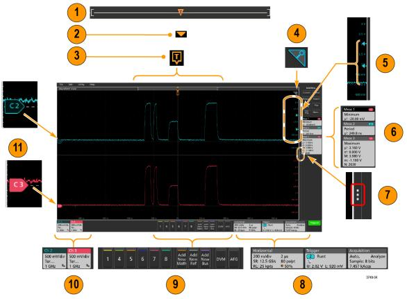
1. The Waveform Record View is a graphical high-level view of the overall waveform record length, how much of the record is on the screen (shown in brackets), the location of key time events including the trigger event, and the current position of waveforms cursors.
