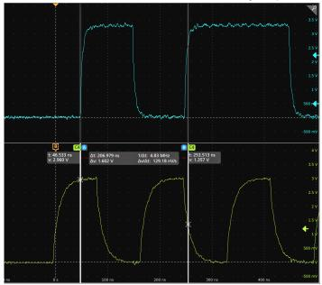
5. To further configure cursors, double-tap on either cursor line or the cursor readouts to open the **Cursors** configuration menu. For example, tap the Cursor type to select the cursors to display, such as Waveform, V Bars, H Bars, and V&H Bars.
