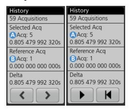
The Reference acquisition readout shows the timestamp when the acquisition occurred in time in history. It also displays the delta between the Selected acquisition and the Reference acquisition timestamps.
