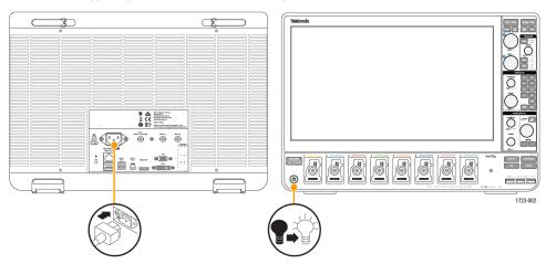
Figure 1: Power cord connector and power standby switch
