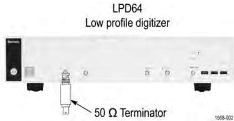
1. Attach a 50  $\Omega$  terminator to the oscilloscope channel 1 input.
