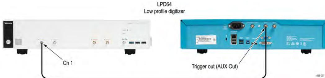
2. Tap **File > Default Setup**. This resets the instrument and adds the channel 1 badge and signal to the display.
