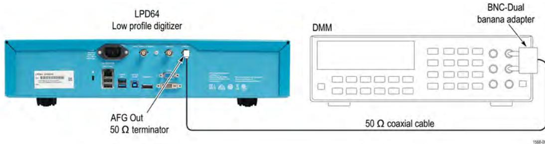
Figure 6: DC offset tests
