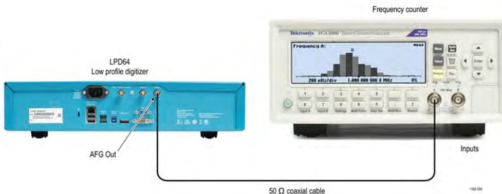
Figure 2: Frequency/period test
