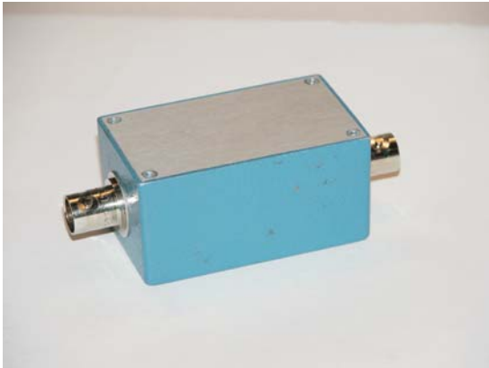
A) Exterior view of filter box
