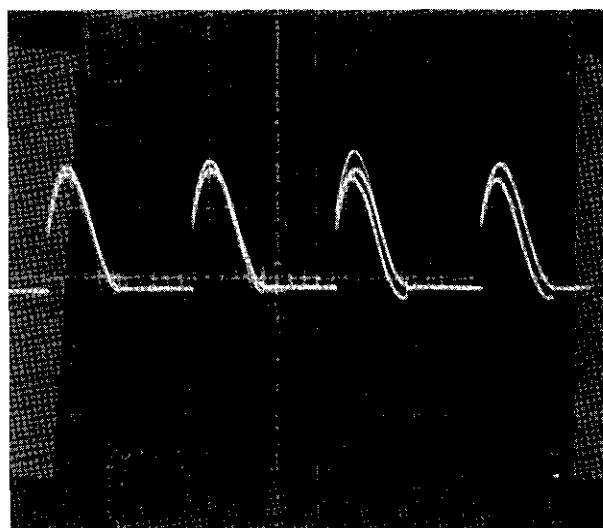
FIGURE 9. Wave Form with R131 Adjusted. A Type 503 Oscilloscope was used; horizontal sweep was 5 msec/cm; vertical, 2 v/cm.
