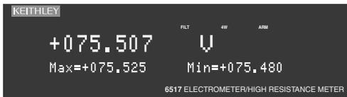
**Maximum and Minimum** — This display shows the maximum and minimum readings that have occurred since the display was entered. Maximum and minimum values are reset by pressing the present function key or by leaving the display.
