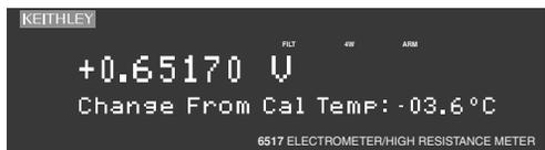
**Change from cal temp** — With temperature readings enabled, this display indicates the difference between the present internal temperature and the internal temperature when the instrument was last calibrated. See Section 1, “External Temperature Measurements,” to enable temperature readings.
