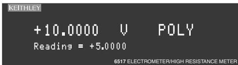
**Calculated and Actual** — This display is used with a math calculation. While the top line provides the result of the math calculation, the bottom line provides the raw reading.
