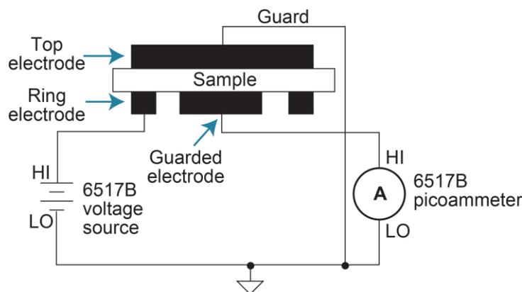
The 6517B automatically performs the following calculation and displays the surface resistivity reading:
