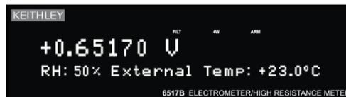
These readings can also be included as data elements for the bus interfaces (GPIB and RS-232) and the buffer.
