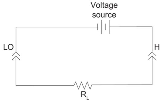
You can also use the voltage source to form the source voltage, measure current configuration, as described in [High-resistance meter connections](#) (on page 3-4).
