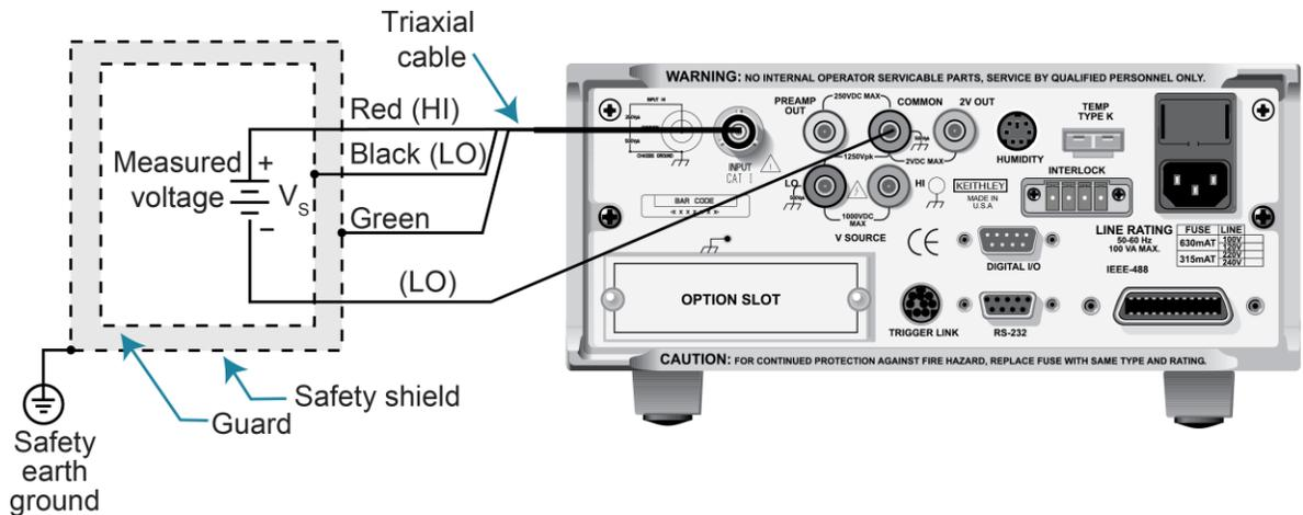
Figure 30: Guarded voltage measurements - equivalent circuit
