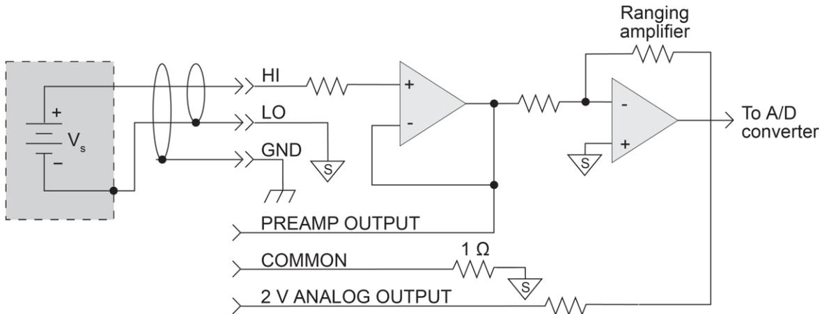
Figure 29: Guard voltage measurement connections
