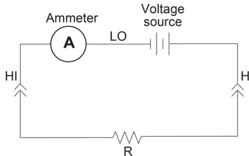
This configuration assumes the **METER-CONNECT** setting is enabled, which internally connects the voltage source LO to ammeter LO.
