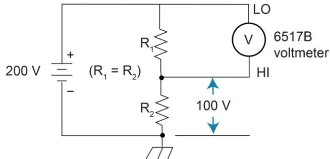
In the following figure, a shock hazard (200 V) exists between the meter input (HI and LO) and chassis ground. If meter input LO is connected to a noise or guard shield, the shock hazard is also present on that shield.
