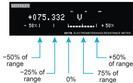
The plus and minus percentage of range that is programmed (0.01% to 99.99%) applies to all functions. Because of rounding, values greater than 99.5% are shown as 100% and, likewise, values greater than 1% (such as 1.67%) are shown rounded to the nearest integer percent.
