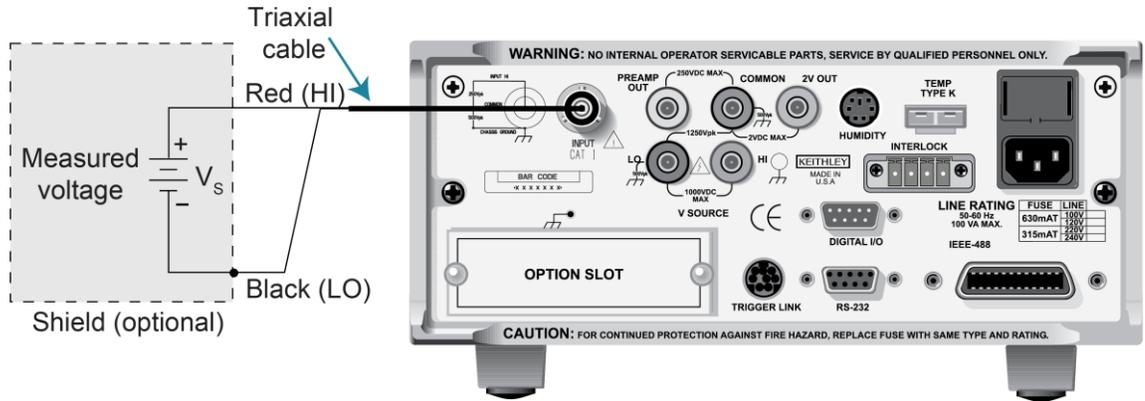
Figure 28: Unguarded voltage measurements - equivalent circuit
