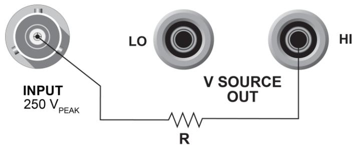
The equivalent circuit for this configuration is shown in the following figure.
