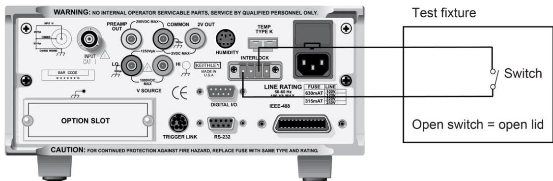
See the following figure for typical connections for resistance measurements to the Model 8009 test fixture.
