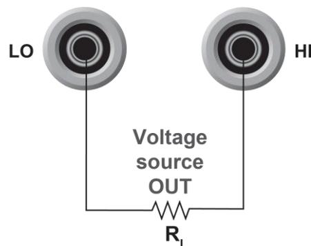
Using these terminals places the independent voltage source in series with the external circuit ( $R_L$ ), as shown in the following figure.
