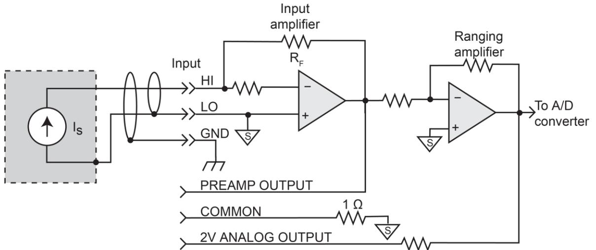
If you are measuring current in a floating circuit where significant leakage may exist between the ammeter input and circuit low, connect the 6517B to the circuit as shown in the following figure. Notice that ammeter input LO is connected to circuit high.
