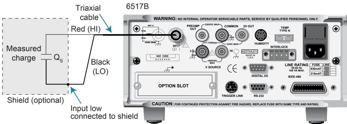
**Figure 42: Typical connections for charge measurements - equivalent circuit**
