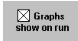
For slow computers, keeping the graphs hidden while the test is in progress helps eliminate timing errors. When a timing error occurs, the Warning Message panel appears (see Figure 2-13). See “Measurement Timing” for more information.
