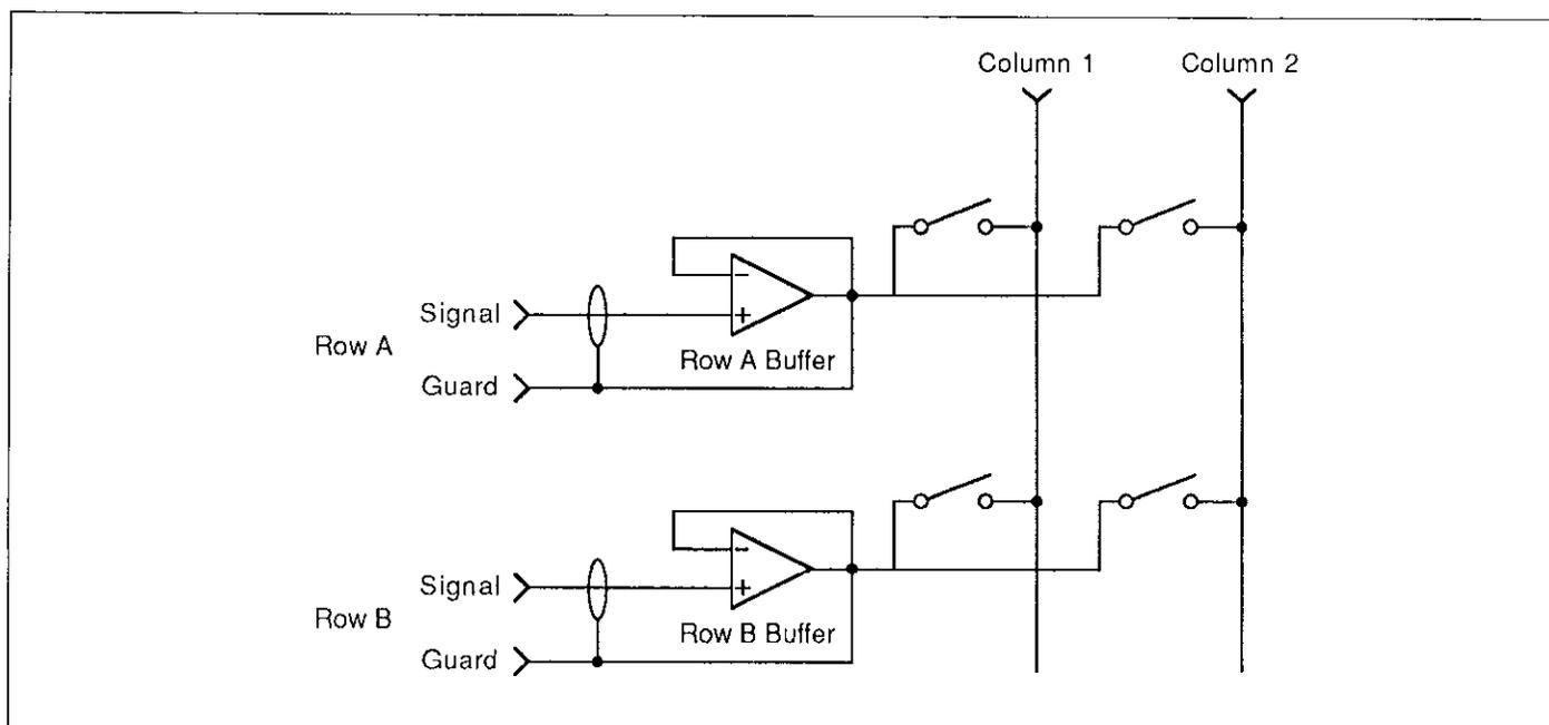
Figure 3-7. Buffer Configuration
