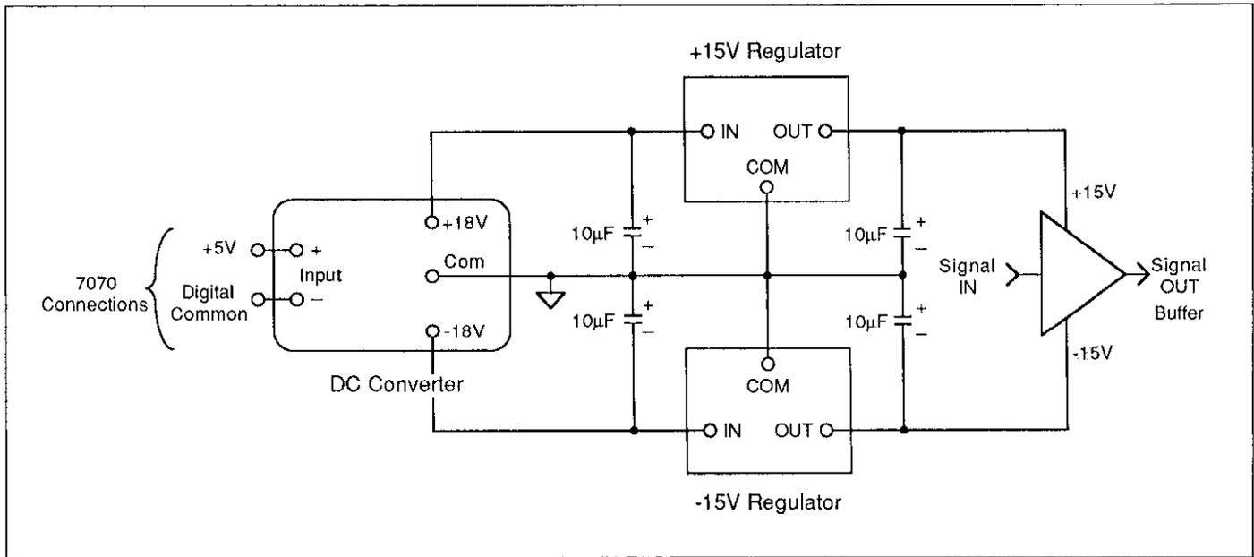
Figure 3-8. DC Converter Used to Power Buffer ICs
