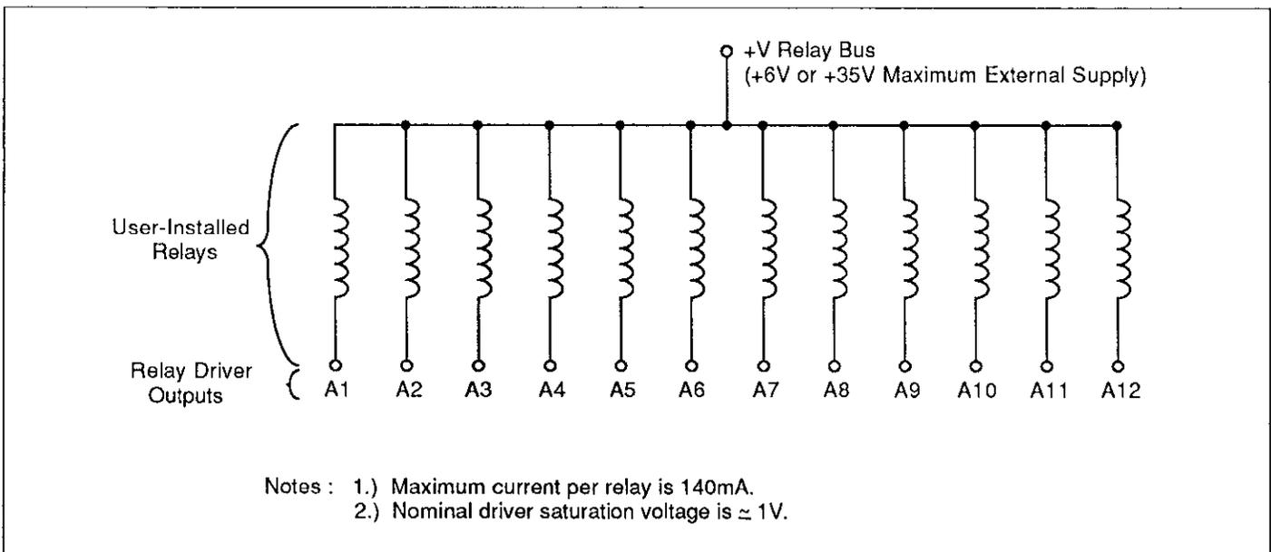
**Figure 2-10. Typical Relay Coil Connections (Row A Shown)**
