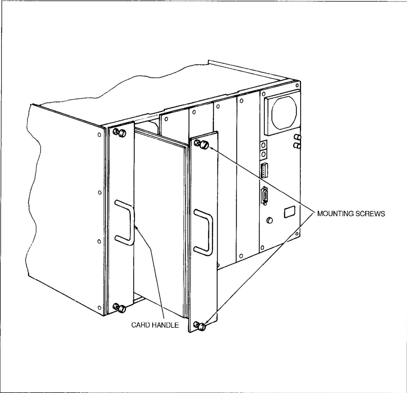
Figure 2-5. Model 7070 Installation
