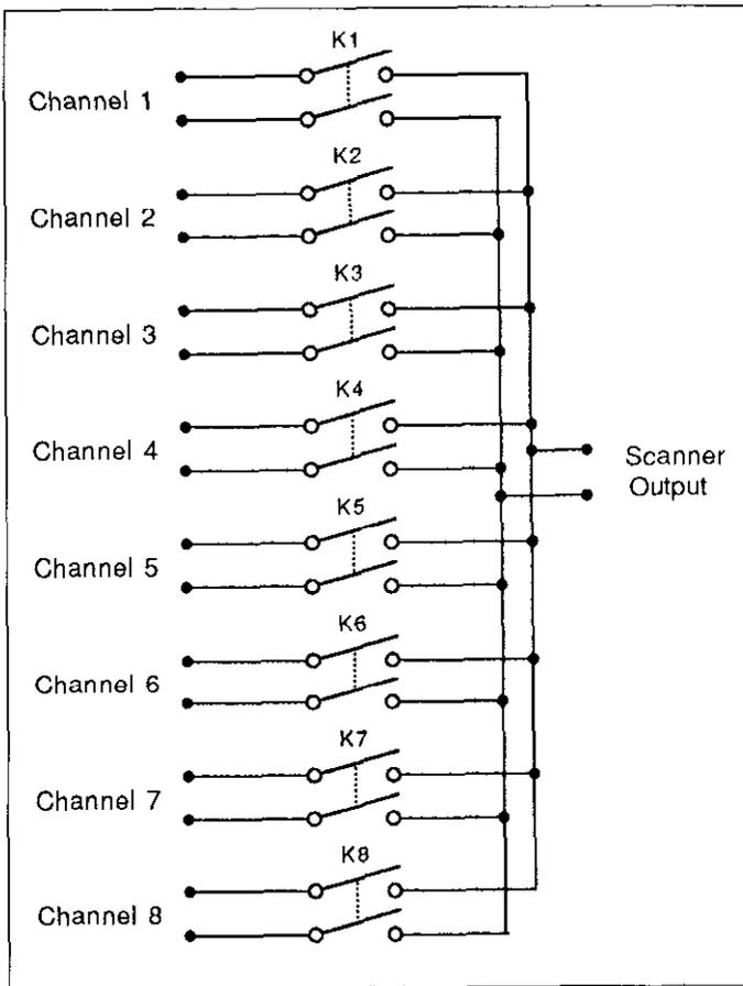
Figure 3-2. 8-Input, 2-Pole Relay Scanner
