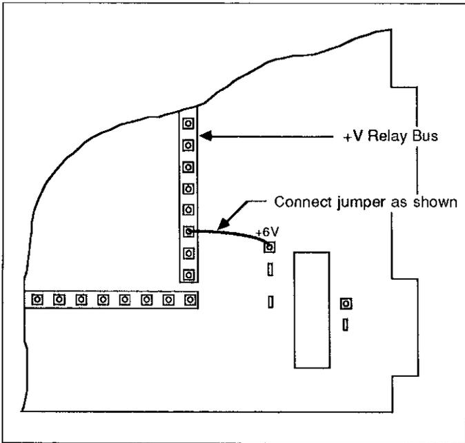
**Figure 2-7. Jumper Installation for Internal Relay Supply**
