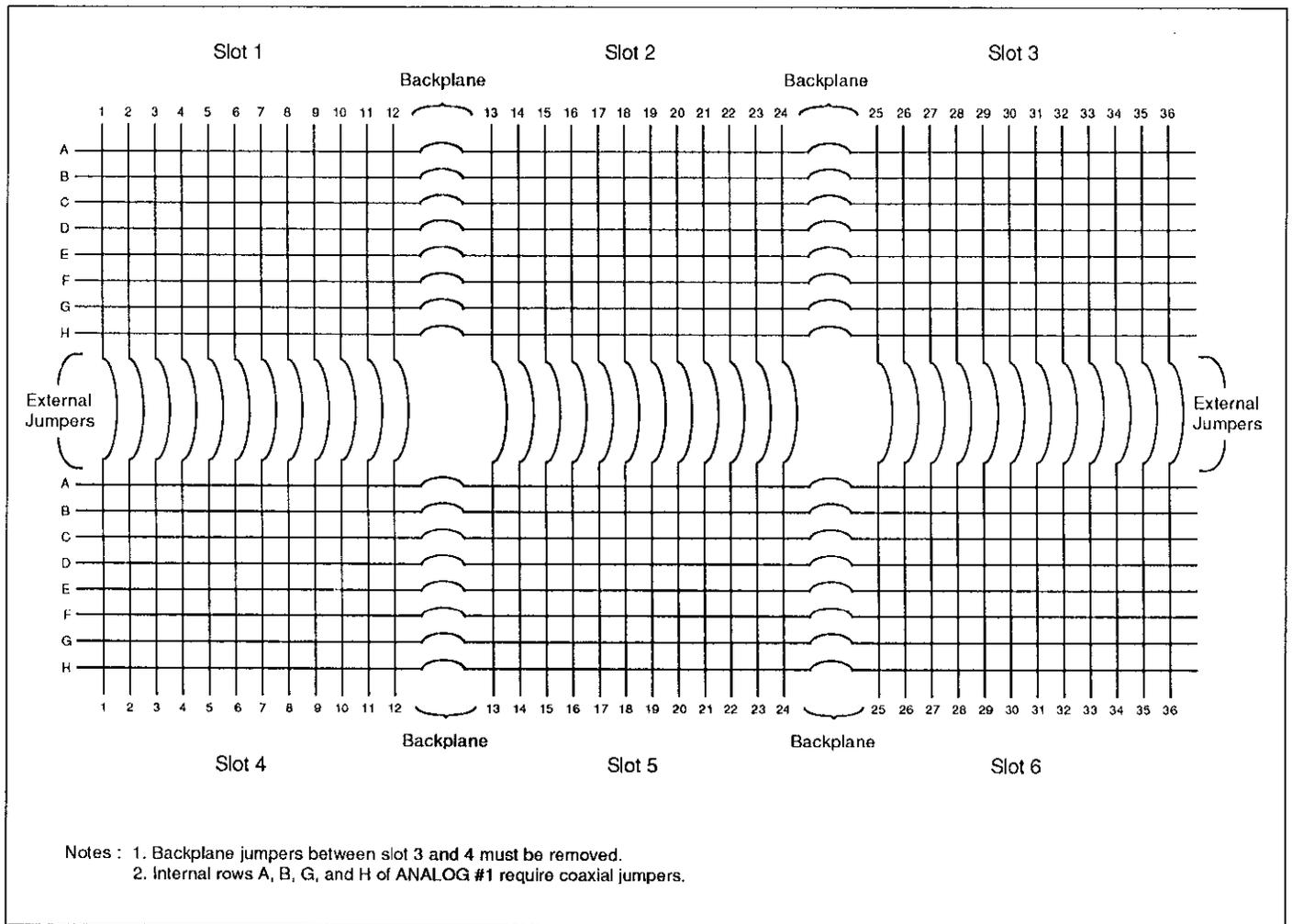
**Figure 2-14. 16 × 36 Matrix Constructed by External Jumpering**
