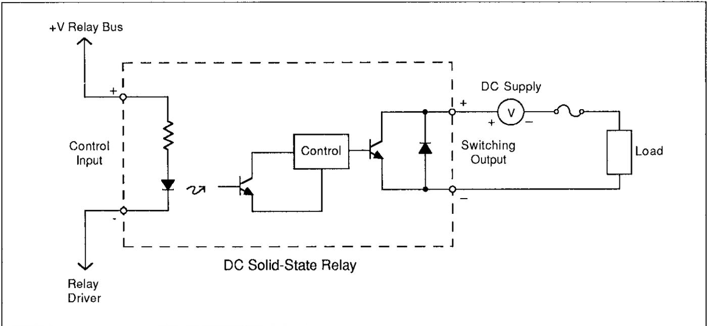
Figure 3-12. Typical DC Solid-state Relay
