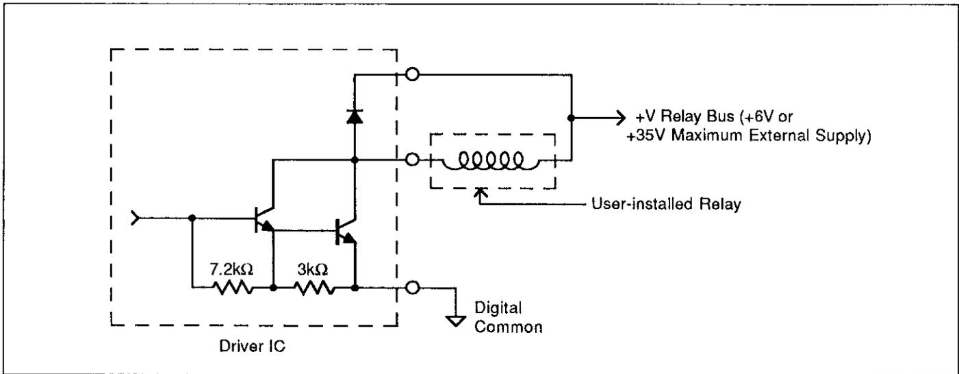
**Figure 2-9. Typical Relay Driver Output**
