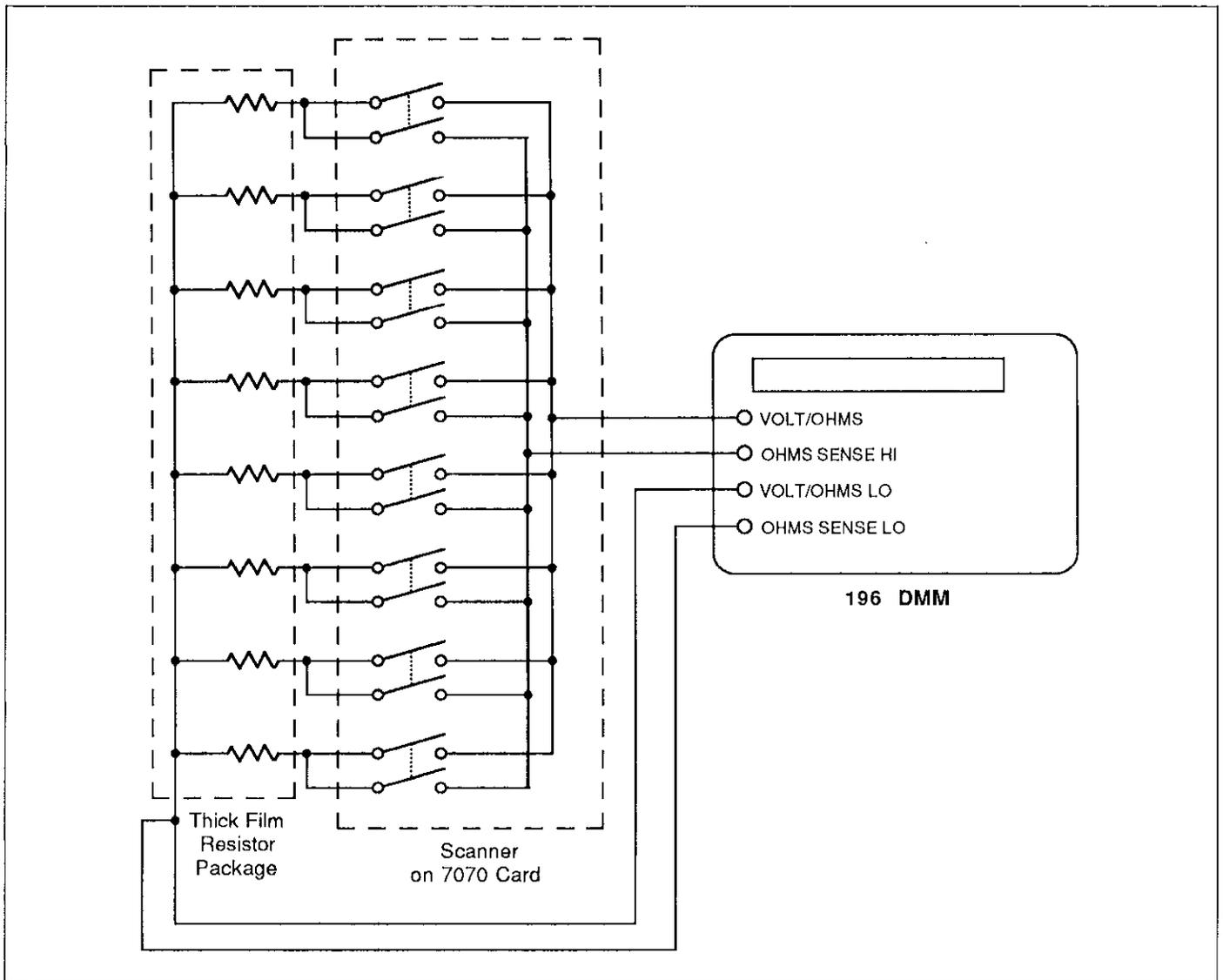
Figure 3-5. Testing Thick Film Resistor with a Scanner
