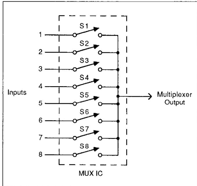
Figure 3-15. Typical Multiplexer IC
