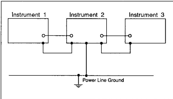
**Figure 2-16. Eliminating Ground Loops**
