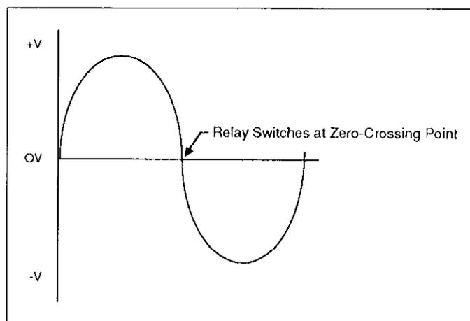
Figure 3-11. Zero-crossing Switching
