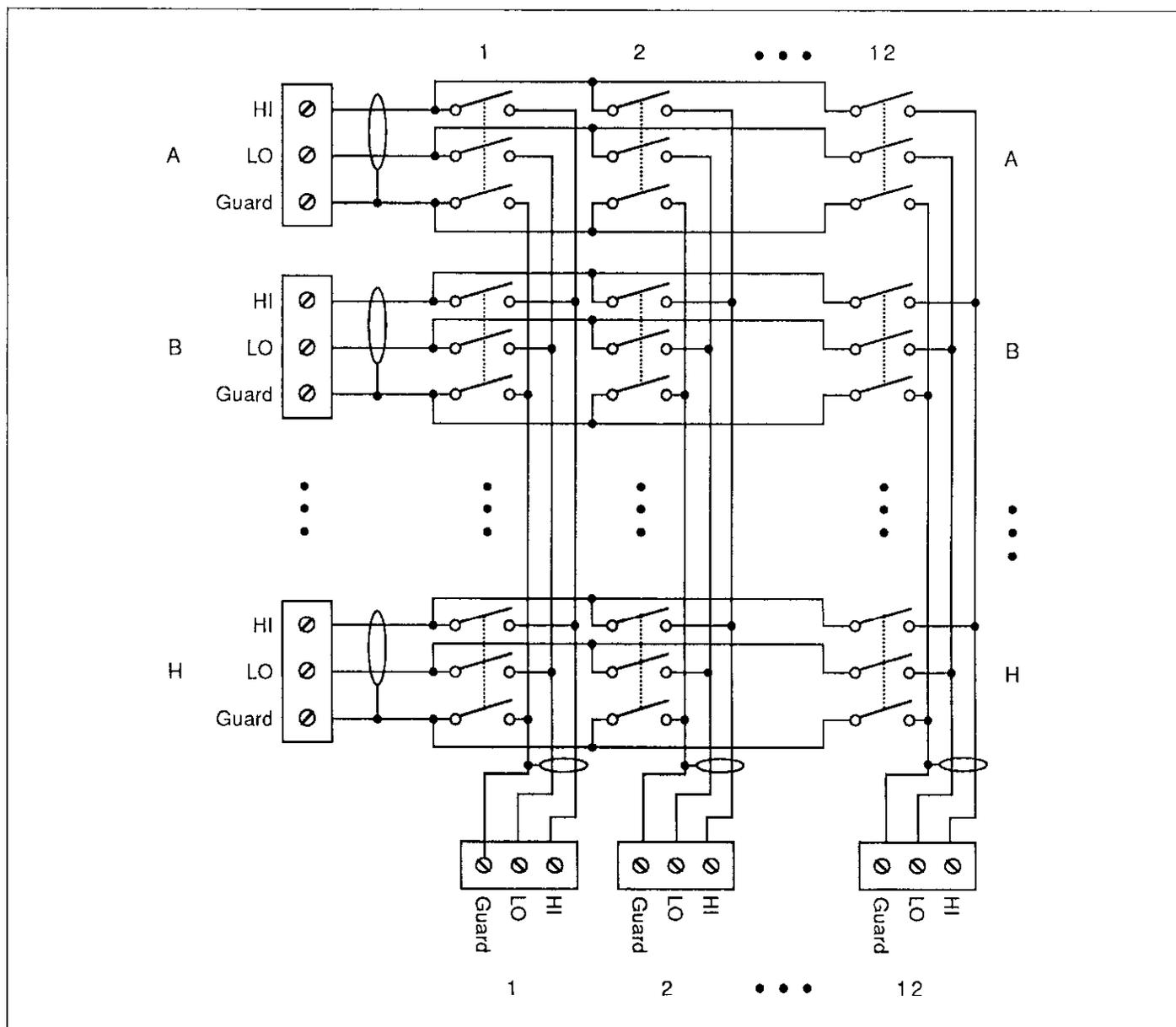
Figure 2-11. Relay Matrix Wiring
