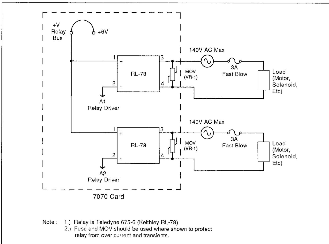
Figure 3-14. Typical Solid-state Relay Application
