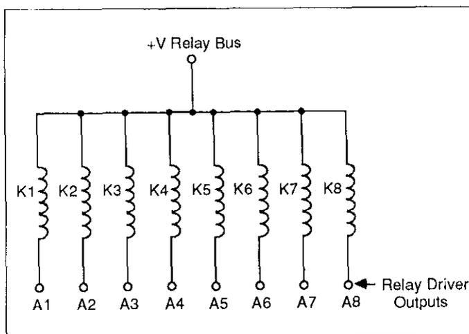
Figure 3-3. Scanner Relay Coil Wiring
