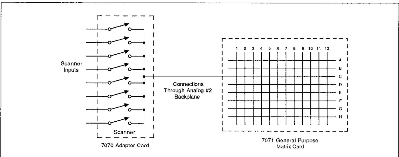
Figure 3-18. Adding a Scanner to a Switching Matrix
