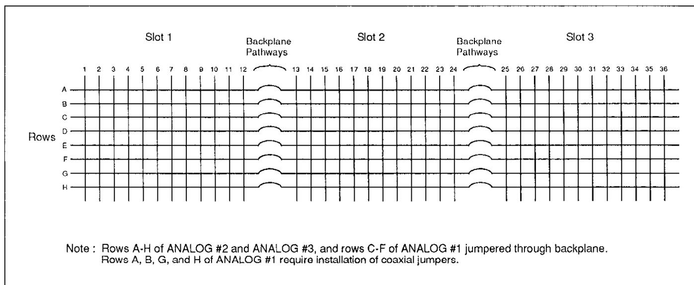
**Figure 2-13. Connecting Three Cards for  $8 \times 36$  Matrix**
