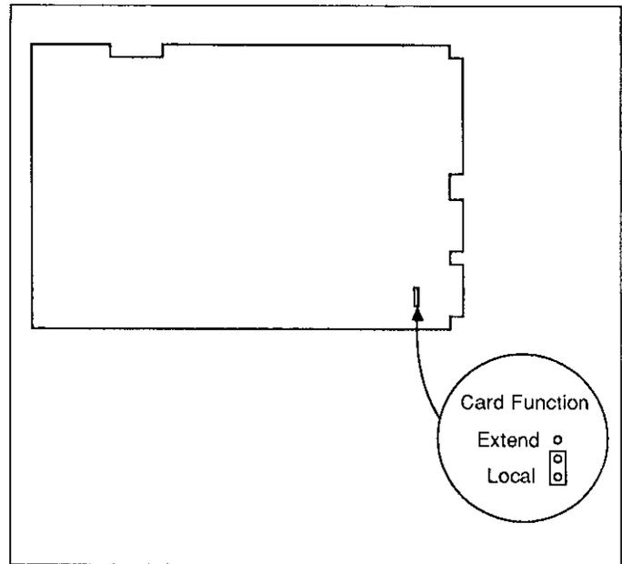
Figure 2-6. LOCAL Function Jumper Position
