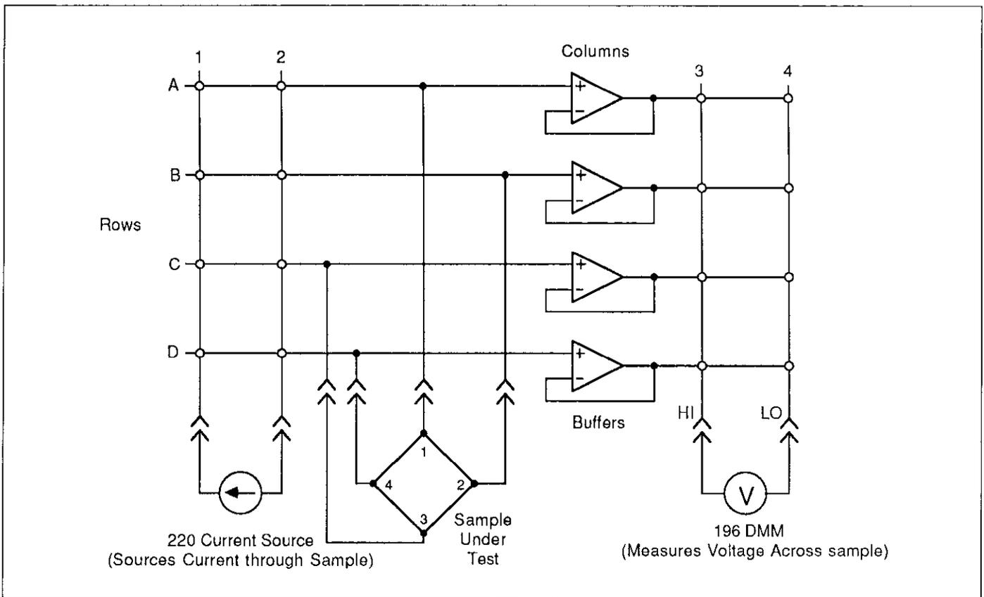
**Figure 3-9. Typical High-Resistivity Test System**
