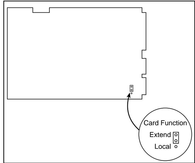
Figure 2-2. Extend Function Jumper Selection
