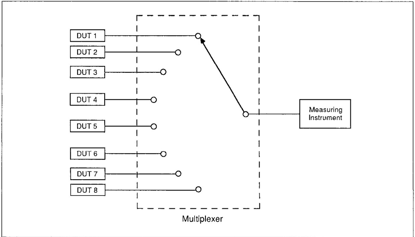
Figure 3-1. A Scanner as a Rotary Switch
