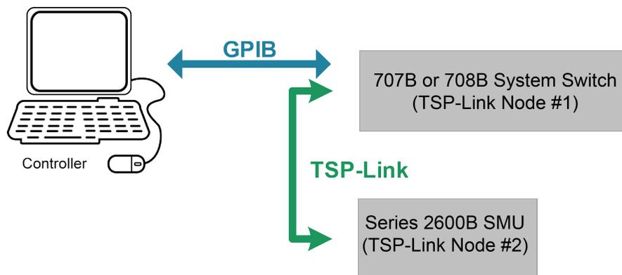
To configure the TSP-Link communication interface, each instrument must have a unique TSP-Link node number. Configure the node number for the Model 707B or 708B to 1 and the SourceMeter Instrument to 2.
