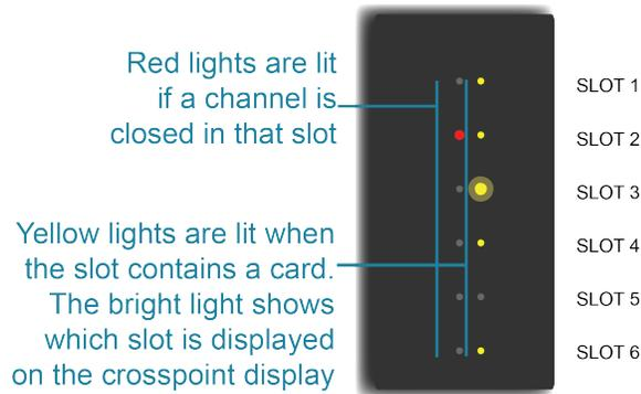
In the figure above, there are cards in five slots, no card in slot 5, and the channels for the card in slot 3 are displayed on the crosspoint display. Also, at least one channel is closed on the card in slot 2.
