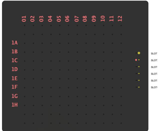
The crosspoint display has a list of slots on the right. To the left of the slot list are lights that show you an overview of the cards in the instrument's slots.
