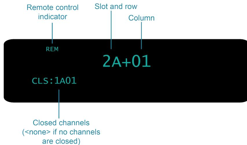
By default, the top line of the display shows the slot, row, and column of the selected channel.
