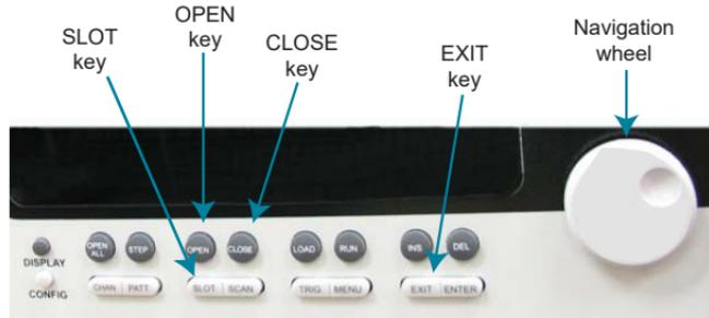
2. Turn the navigation wheel to display the firmware version information for the installed switching cards.
