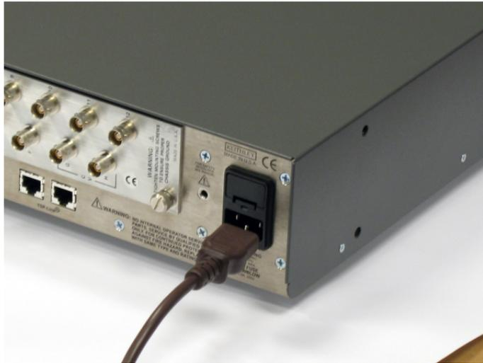
3. Connect the plug of the power cord to a grounded AC outlet.
