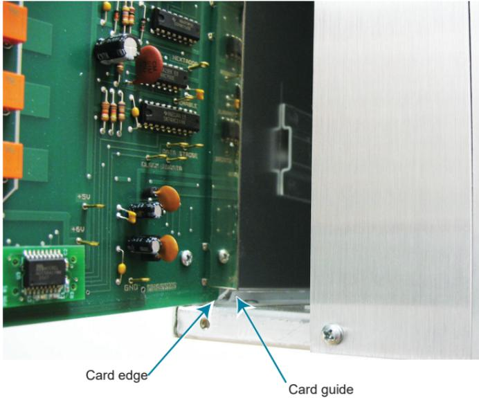
6. Slide in the card. For approximately the last ¼ inch, press in firmly to mate the card connector to the 707B or 708B connector.
