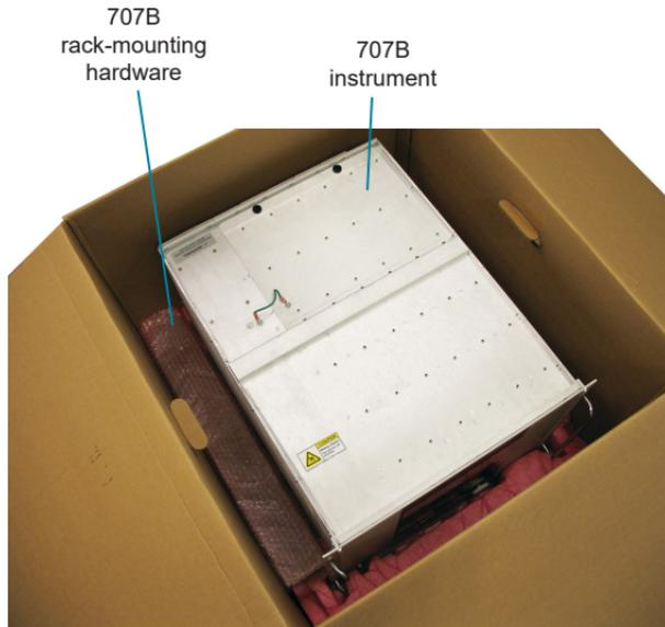
7. Inspect the instrument for any obvious signs of physical damage. Report any damage to the shipping agent immediately.
