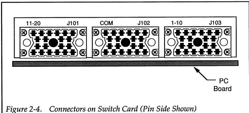
Figure 2-4. Connectors on Switch Card (Pin Side Shown)
