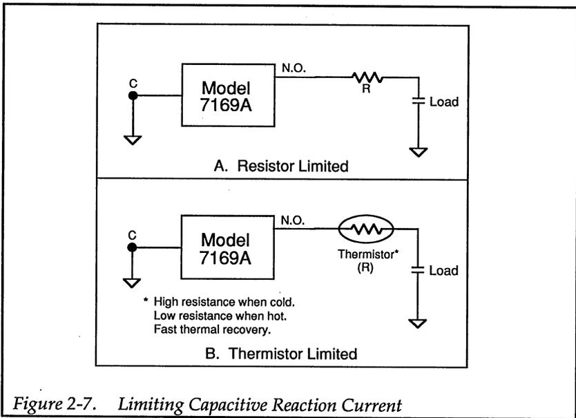
Figure 2-7. Limiting Capacitive Reaction Current
