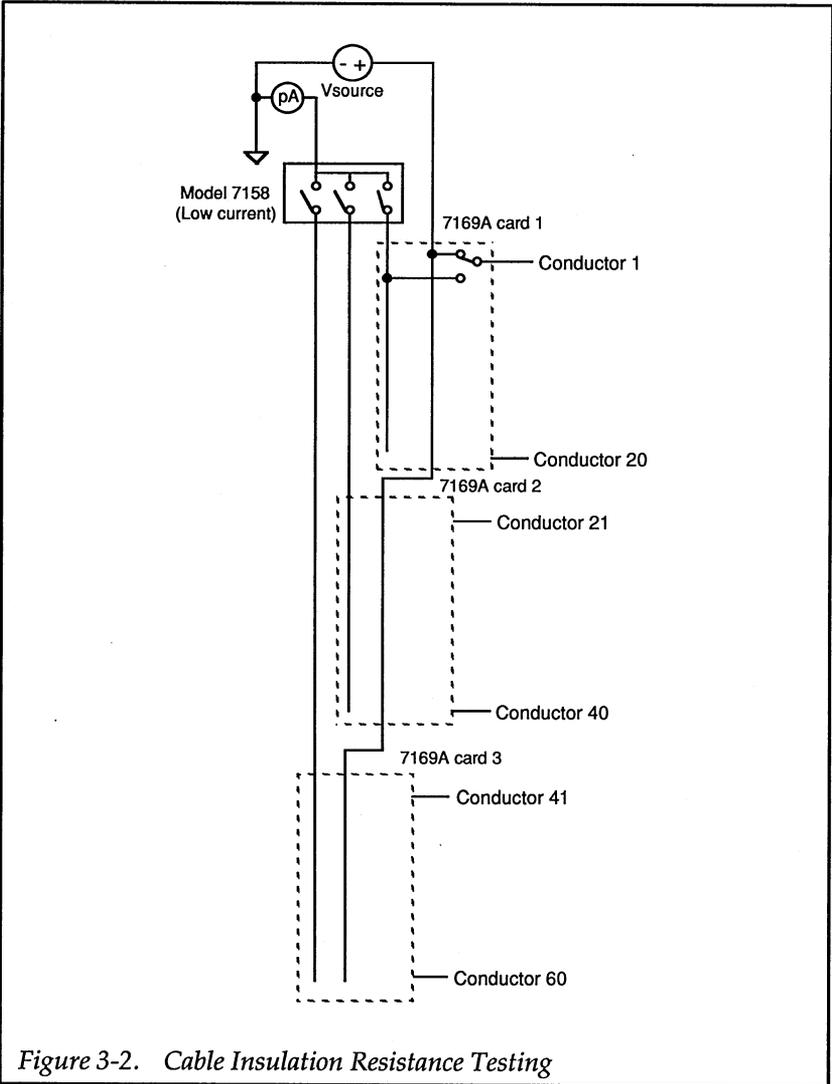
Figure 3-2. Cable Insulation Resistance Testing
