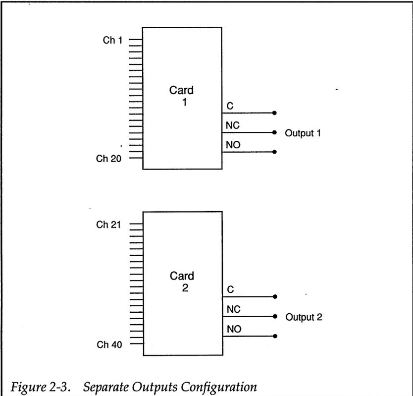
Figure 2-3. Separate Outputs Configuration
