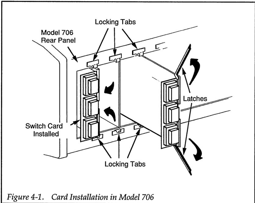
Figure 4-1. Card Installation in Model 706
