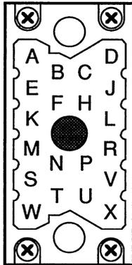
Figure 2-5. Female Connector Pin Identification
