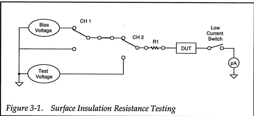
*Figure 3-1. Surface Insulation Resistance Testing*
