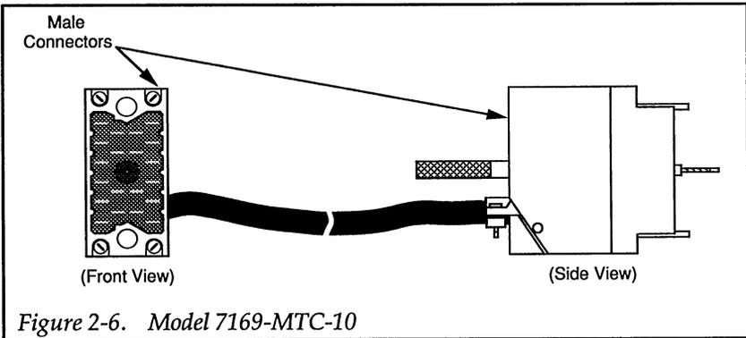
If the cable is to be used, a 7169-MTR becomes part of the user's test fixture with instrumentation and DUTs crimped directly to its terminal pins. The Model 7169-MTR is the same connector that is used on the panel of the Model 7169A. Its pins will accommodate up to #18 AWG wire.
