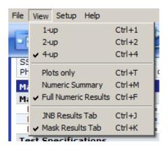
The summary selections list the noise and jitter measurements but not the breakdown of the measurements. The two results tabs select relevant jitter or mask test results.
