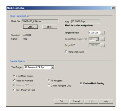
**NOTE.** Changes to mask test settings are reflected in the current plots and results.
