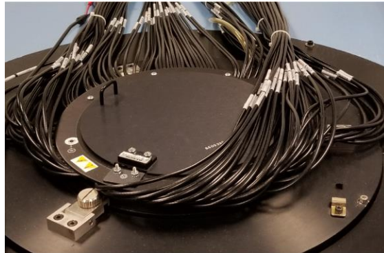
Figure 15: PCA cable routing example
