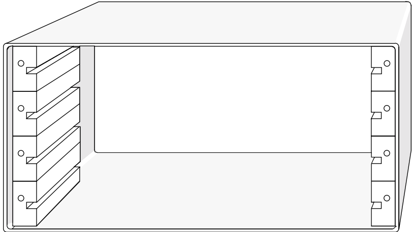
Figure 3-7. ENCL-4 Enclosure with Four Pairs of Slotted Card Guides (rear panel not shown)
