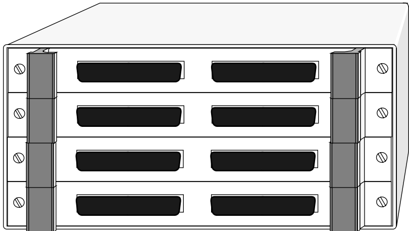
Figure D-1. ENCL-4 Enclosure with Four EXP-1800s Installed
