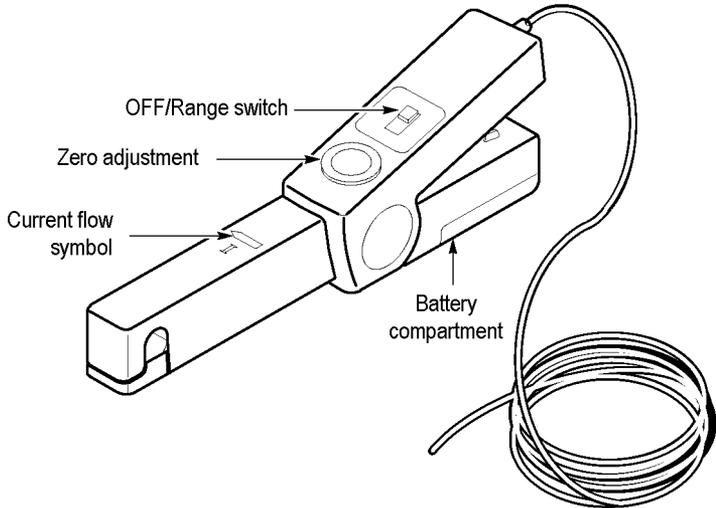
**Figure 1: A622 AC/DC Current Probe**
