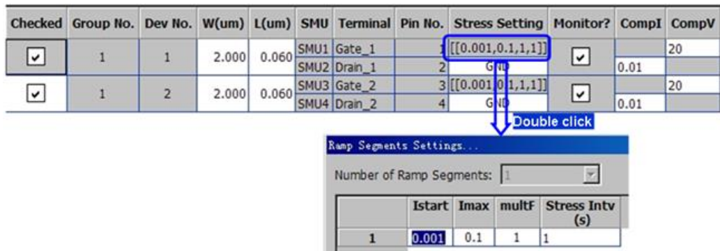
Figure 83: Device and SMU settings for JRamp/TDDb_CCS
