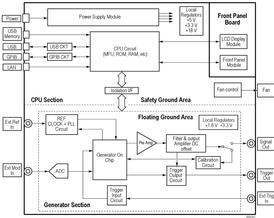
Figure 3: Block diagram
