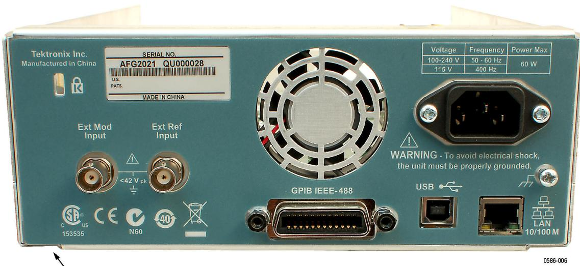
Use screw driver or tweezers to lift label from the rear panel
