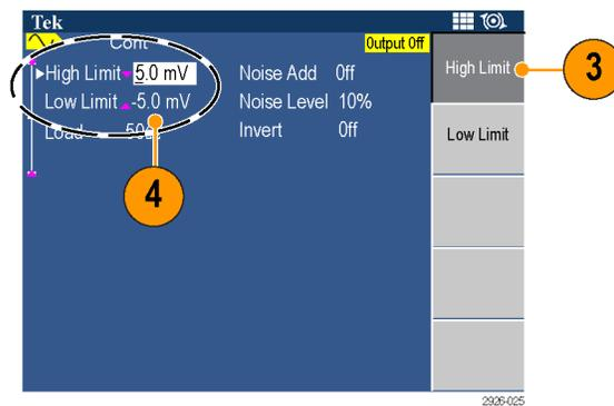
5. Use the numeric keys or the general purpose knob to set the High Limit to 50 mV and the Low Limit to -50 mV.
