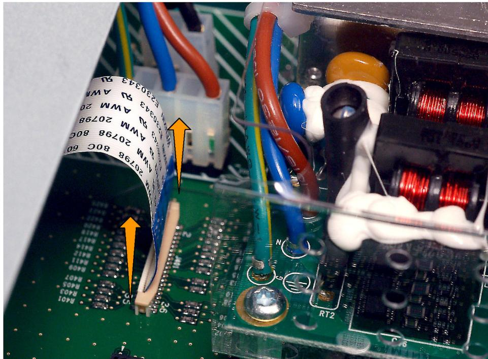
Lift both sides of connector tab
