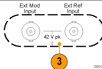
**WARNING.** To avoid personal injury due to electric shock, do not apply voltages in excess of 42 Vpk to any BNC connector ground or to the chassis ground.
