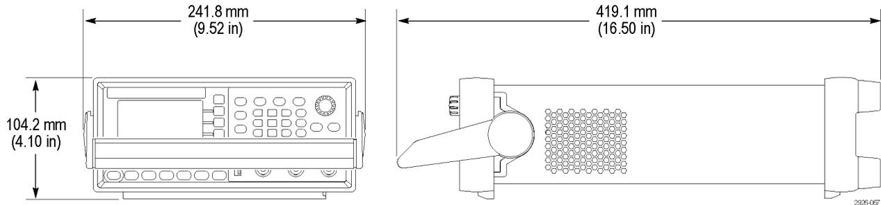
Figure 1: Instrument dimensions
