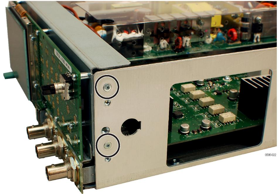
**Figure 16: Location of the front chassis retaining screws**
