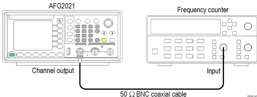
**Figure 4: Frequency/Period tests**
