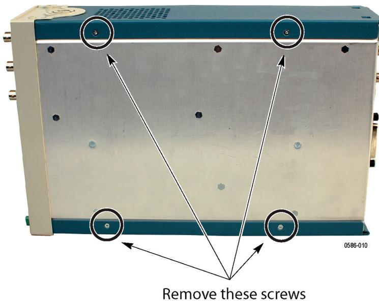
**Figure 7: Location of the case retaining screws**
