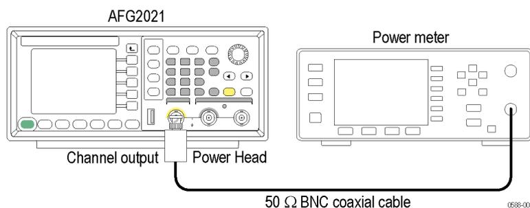
**Figure 5: Flatness adjustment connections**
