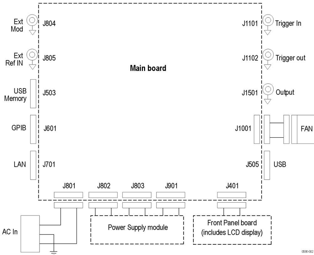
**Figure 30: Interconnections for the AFG2021 (GPIB and LAN only on AFG2021 with Option GL)**
