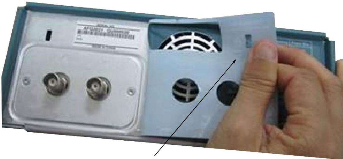
After the label is lifted, use thumb and index finger to carefully peel label from rear panel
