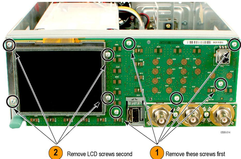
Figure 13: Removing the Front Panel board
