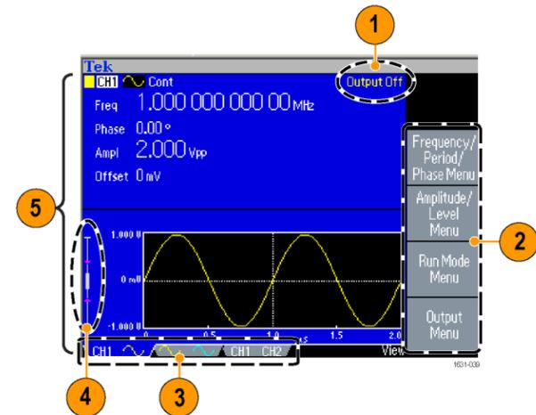
1. **Output status:** If the output is set to disable, Output Off message is displayed in this area. When you push the front panel channel output button to enable the output, the message will disappear.
