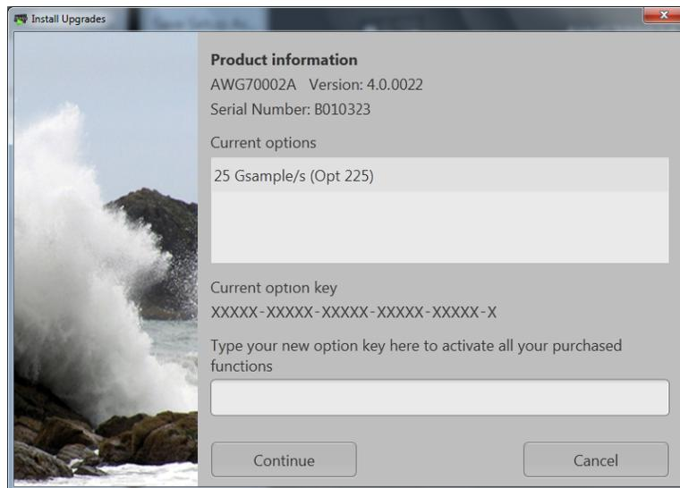
6. Enter the option key provided by Tektronix, and follow the on-screen instructions to install the option.
