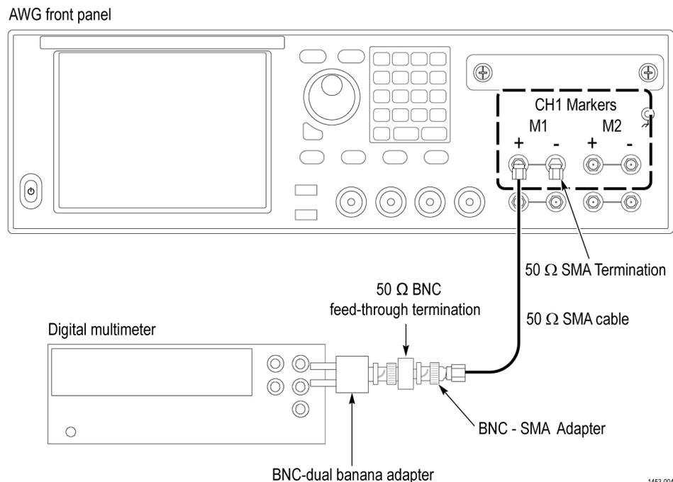
Figure 15: Equipment connection to verify the marker high and low level accuracy
