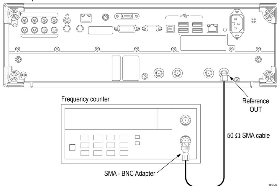
Figure 12: Equipment connection to verify the 10 MHz reference frequency accuracy
