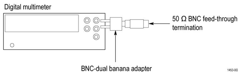
**Figure 13: Equipment connection for measuring the termination resistance**
