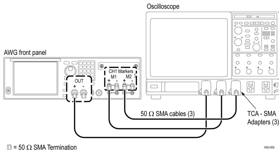
Figure 4: Equipment connections to check the analog and marker outputs
