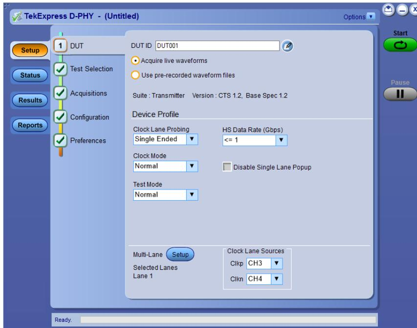
The Tektronix TekExpress® D-PHY (Opt. 6-CMDPHY / DPHY12) offers a complete physical layer test solution for transmitter conformance and characterization as defined in the MIPI D-PHY v1.2 specification. The TekExpress® D-PHYTX automated test solution, along with a Tektronix 6 Series / MSO/70K oscilloscope, provides an easy way to test, debug and characterize the electrical and timing measurements of D-PHY data links.
