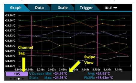
Figure 38: DAQ6510 scanning and temperature graph
