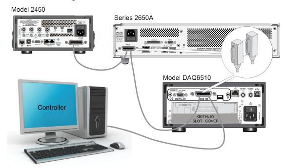
Figure 24: DAQ6510 instrument GPIB connections
