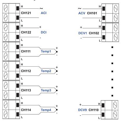
Figure 42: 7700 channel connections
