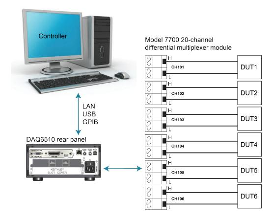
Figure 39: DAQ6510 connections for low-level DCV measurements
