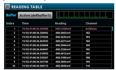
Figure 43: DAQ6510 reading table mixed function multichannel scanning
