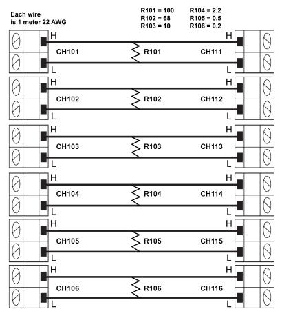
Figure 41: Schematic of 4W measurement
