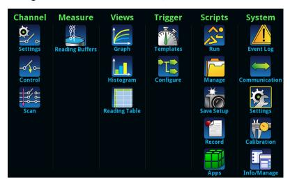
The main menu includes submenus that are labeled in green across the top of the display. Selecting an option in a submenu opens an interactive screen.
