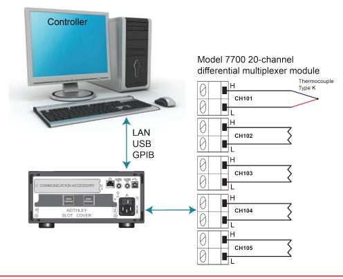
Figure 45: DAQ6510 prescan monitor device connections
