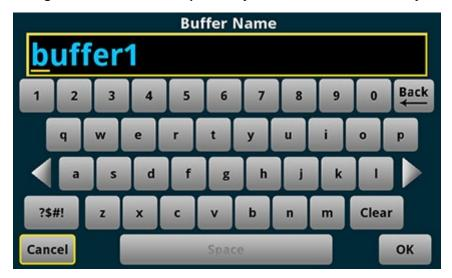
Figure 3: DAQ6510 front-panel keyboard for information entry
