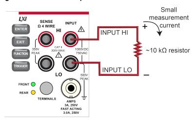
Figure 30: DAQ6510 front-panel 2-wire resistance measurement
