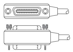
To allow many parallel connections to one instrument, stack the connectors. Each connector has two screws on it to ensure that connections remain secure. The figure below shows a typical connection diagram for a test system with multiple instruments.
