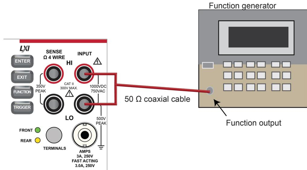
3. Set the function generator output impedance to high, amplitude of 5 V<sub>RMS</sub>, waveform to square wave.
