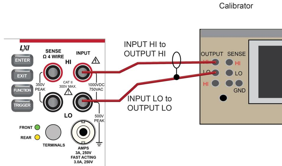
2. On the DMM6500, press the **FUNCTION** key, select the **Digitize Functions** tab, and select **Digitize Voltage**.
