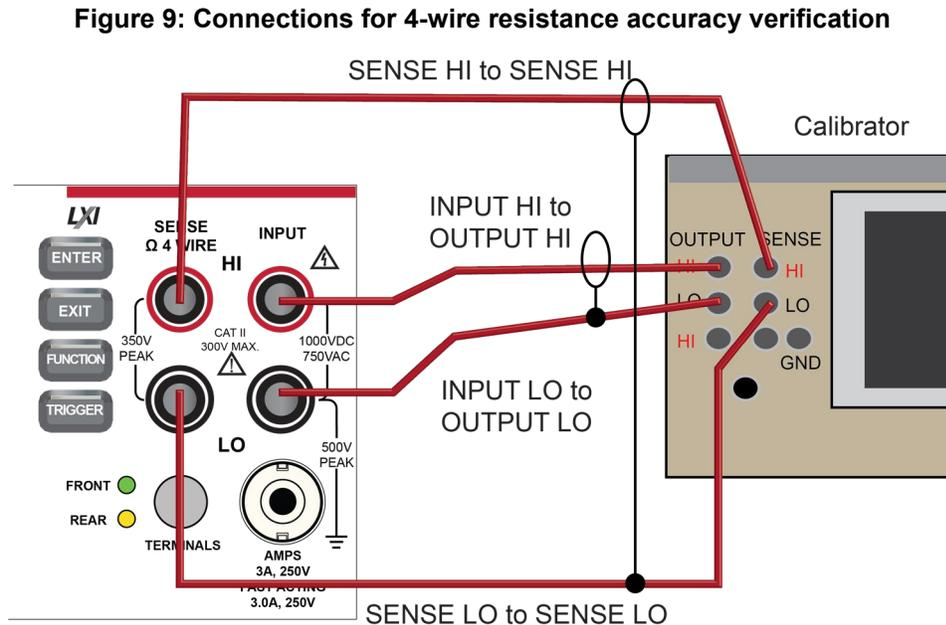
2. Set the calibrator for 4-wire resistance with external sense on.
