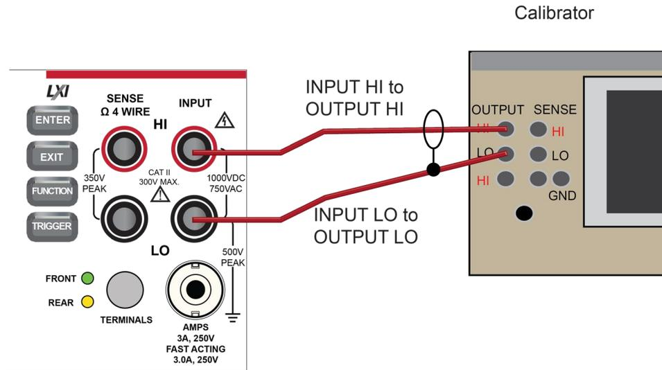
2. On the DMM6500, press the **FUNCTION** key and select **AC voltage**.
