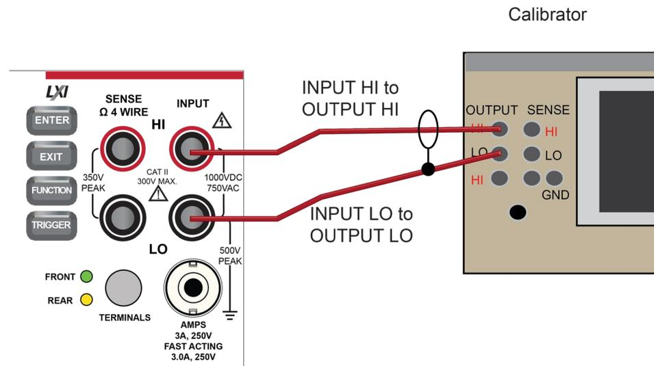
3. Allow the instrument and cables to settle for 30 seconds.
