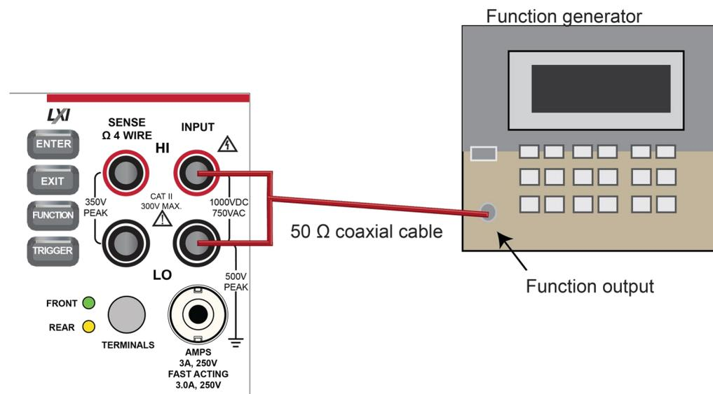
2. On the DMM6500, press the **FUNCTION** key, select the **Measure Functions** tab, and select **Frequency**.
